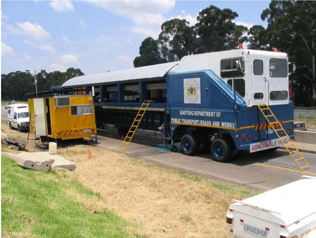
**FIGURE 1 HVS located on a test site.**
