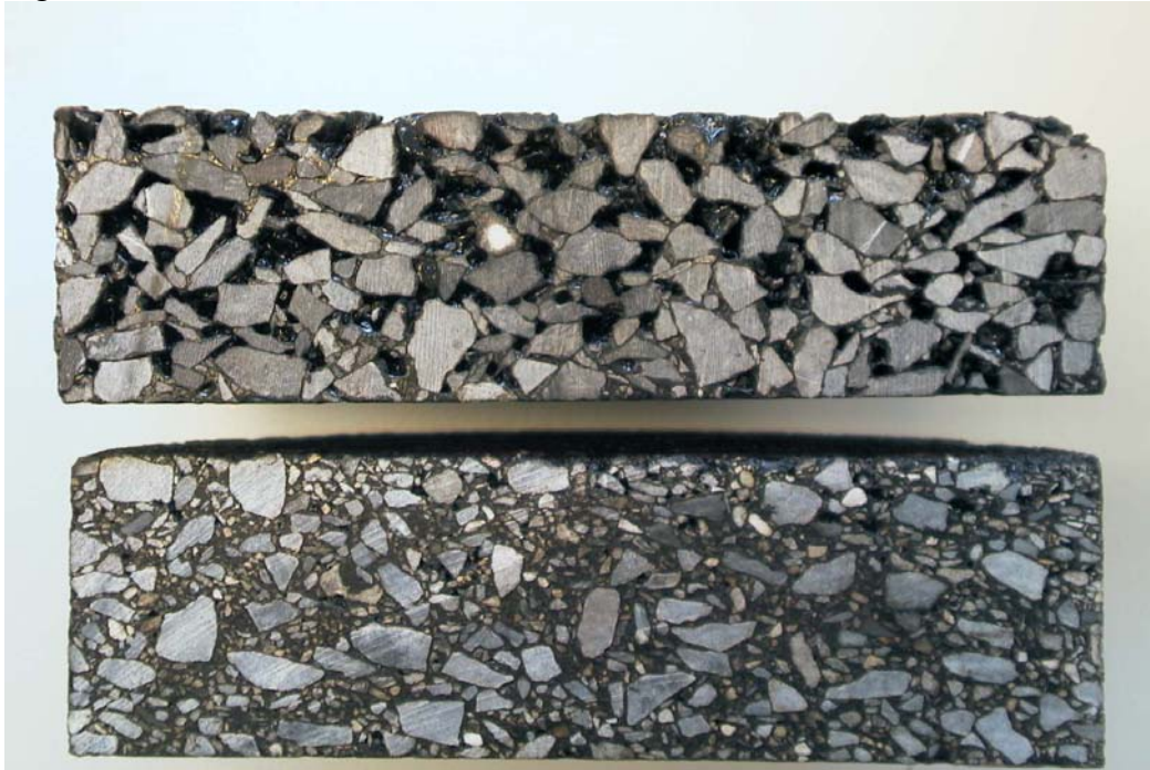
Figure 24: Interconnected Voids of Porous Asphalt
