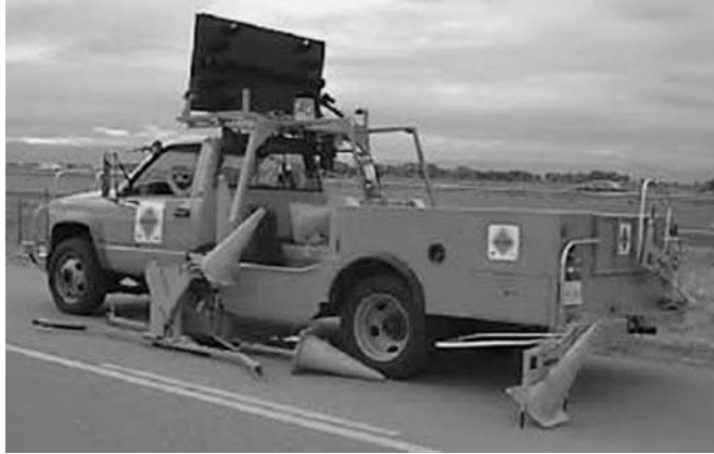
Figure 18 Automatic cone setting device (Source: Advanced Highway and Construction Technology).
