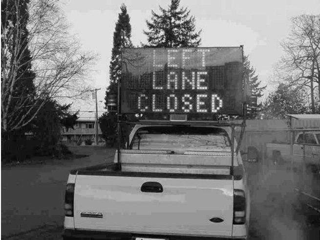
Figure 17 Portable changeable message sign (Source: Washington State DOT).
