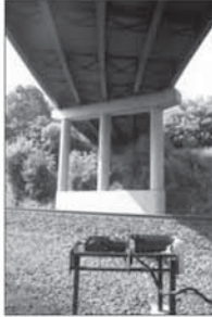
Laser System Measuring Full-Sized Steel Bridge Girders
