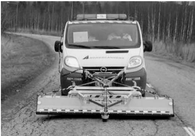
3-D GPR system (Source: Roadscanners, Inc., Finland).
