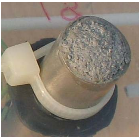
FIGURE 4 The sensor showing the stainless steel counter electrode (CE) and the mortar. The working electrode (WE) is a 3-mm-diameter steel disc, placed concentrically with the CE; the surface of the WE is located about 0.6 cm below surface of the mortar.
