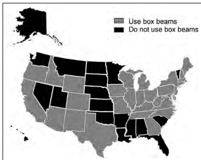
FIGURE 5 Usage of box beam bridges by state.
