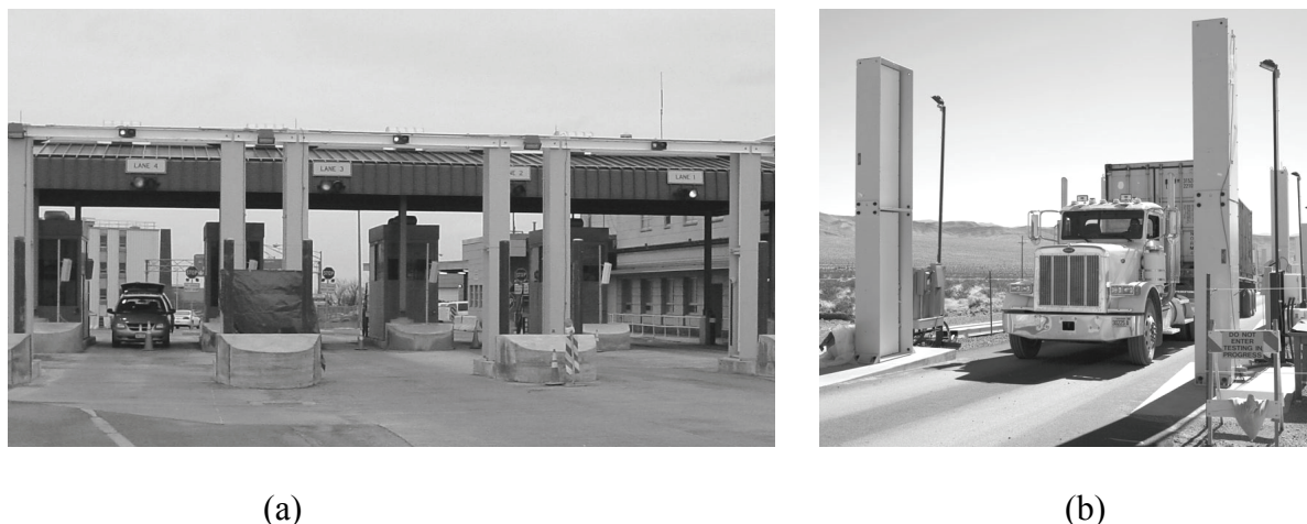
Figure 1.1 (a) The tall pillars closest to the foreground in this photograph are RPMs at a land border crossing between Canada and New York. (b) A truck is shown passing through a series of RPMs and ASPs on a test track. SOURCE: CBP (2008).
