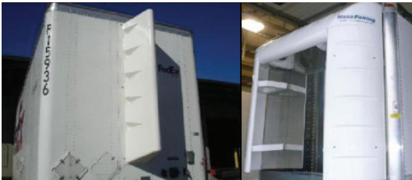
FIGURE 5-13 Laydon vortex stabilizer (left) and nose fairing (right). SOURCE: Courtesy of Laydon Composites.
