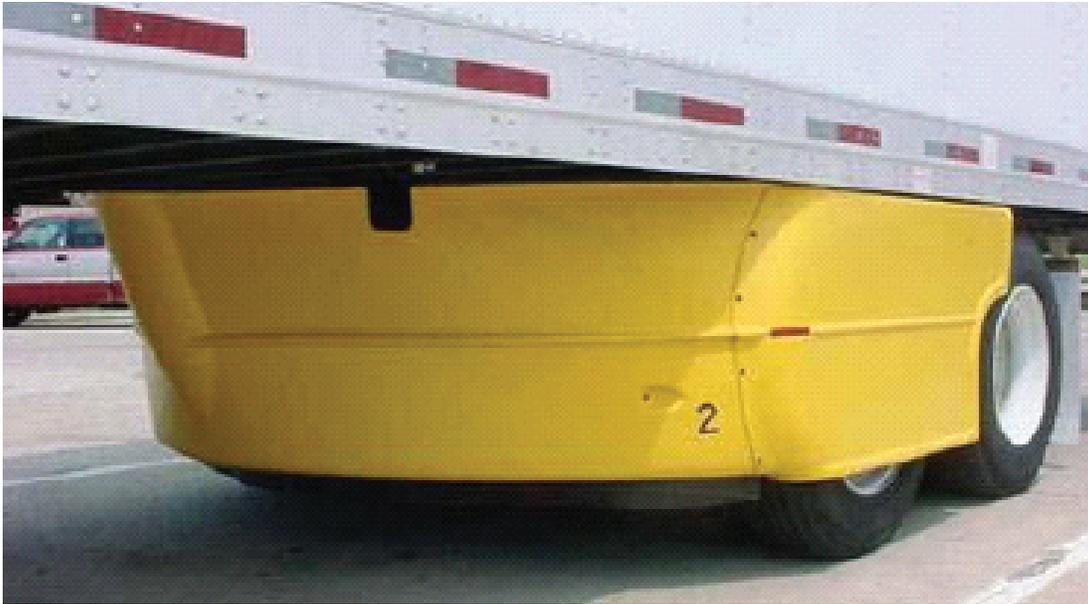
FIGURE 5-14 Trailer bogie cover. SOURCE: TMA (2007).
