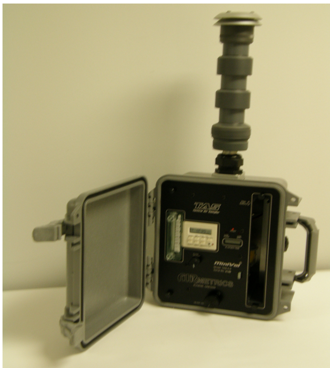
FIGURE 2-2 Assembled MiniVol sampler. Photo courtesy of Philip Hopke, 2009.
