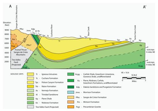
**FIGURE 2.6** West-to-east cross section (see location A–A' in Figure 2.5a) through the Raton Basin shows an asymmetry similar to the San Juan Basin. The primary coal-bearing and CBM-producing units are the Vermejo and Raton formations. Depth to the methane-bearing Vermejo Formation coal zone is about 2,400 feet (Johnson and Finn, 2001). SOURCE: Adapted from Stevens et al. (1992). Reproduced by permission of the Gas Technology Institute.
