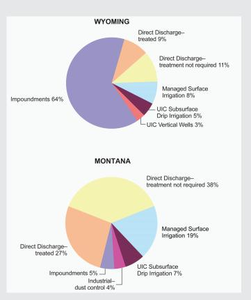
**FIGURE** Proportional representation of CBM produced water management strategies in the Wyoming and Montana portions of the Powder River Basin. The total amount of water produced in the Wyoming Powder River Basin from CBM extraction in 2008 was approximately 678 million barrels. See also Table 2.1 and Figure 2.8.
