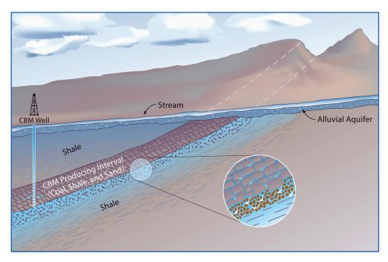
**FIGURE 5.4** Conceptualized schematic showing potential hydrological connection between CBM well, water within CBM bearing aquifers, and surface water. SOURCE: Colorado Geological Survey, available at geosurvey.state.co.us/Portals/0/CBM-SJB-diagramweb2.jpg.
