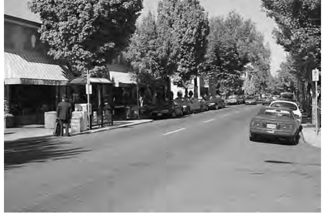
FIGURE 20 Curb extension treatment—Portland, Oregon [Source: TCRP Report 118 (5) ].
