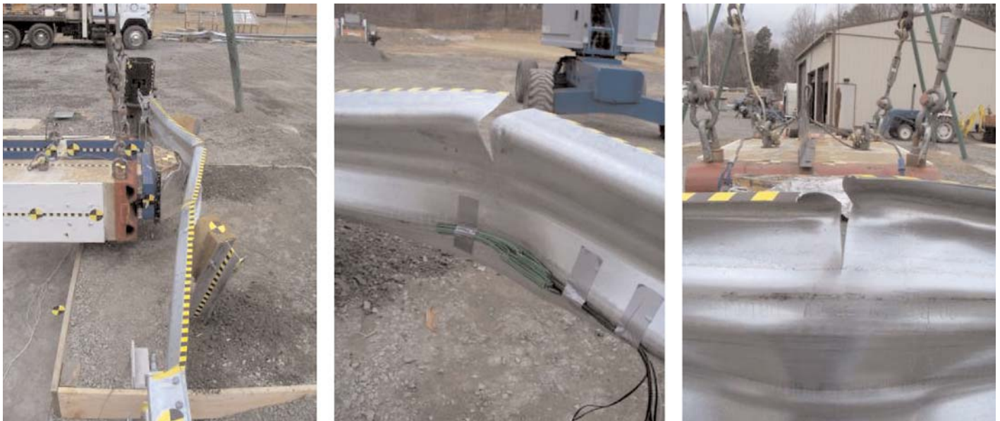
Figure 18. Test 08-2: overall damage (left) and detail views of the additional tearing caused by the pendulum impact (center), and post damage at splice location (right).
