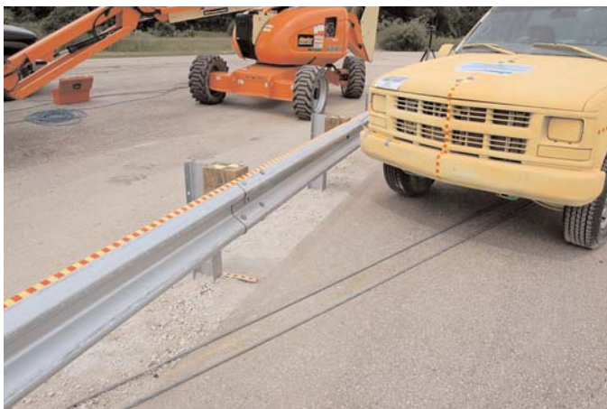
Figure 8. Vehicle orientation prior to first MGA crash test.
