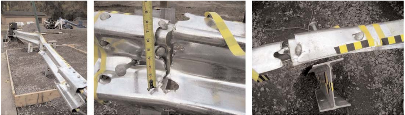
Figure 33. Test 01-4: overall damage (left), rail tear at splice (center), and post damage at splice location (right).
