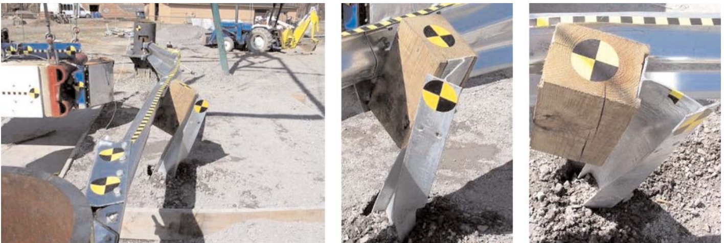
Figure 15. Test 03-2: overall damage (right) and post damage at splice (center) and non-splice location (right).
