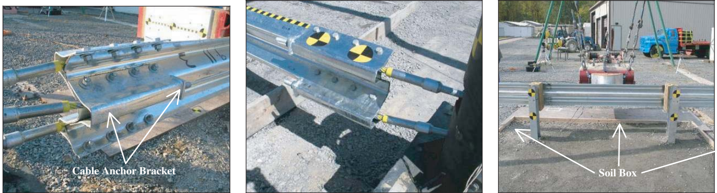
Figure 5. Three cable (left) and two cable (center) w-beam end fixture and soil box (right).
