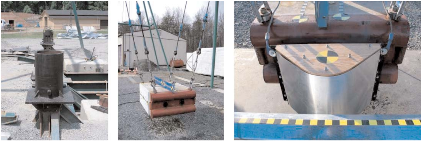
Figure 3. Existing rigid posts (left), FOIL pendulum mass (center), and new impactor face (right).
