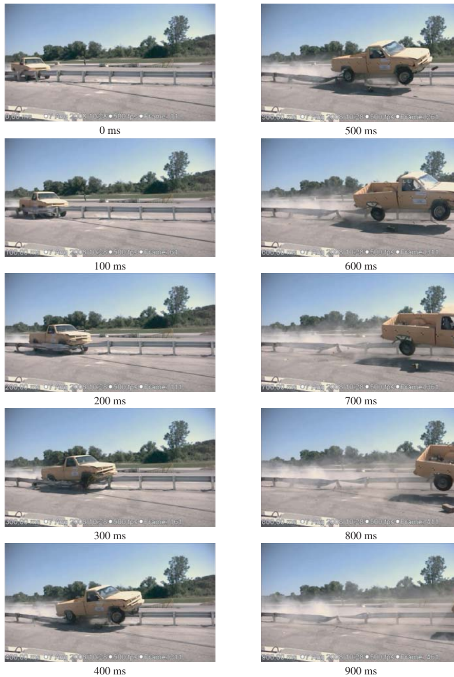
Figure 39. Time series for second, high-speed impact into damaged guardrails.
