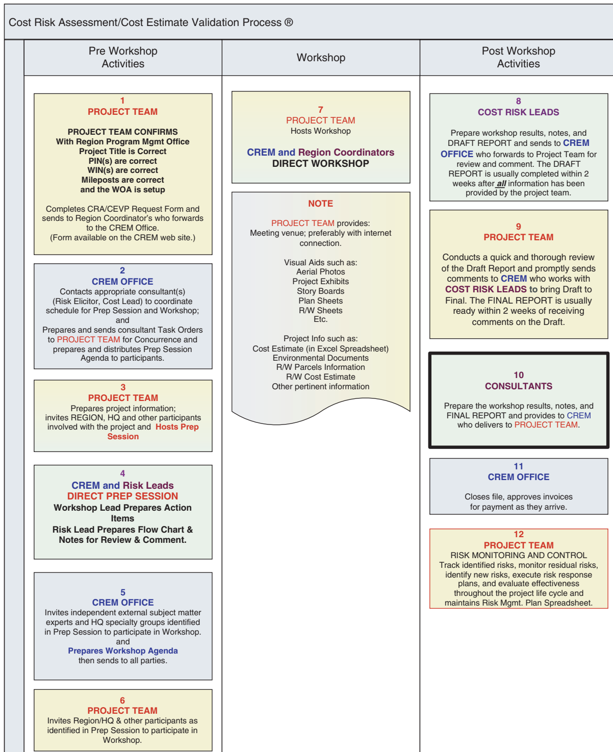
Figure R3.6-1. Example of WSDOT cost risk analysis/cost estimating validation process workshop.
