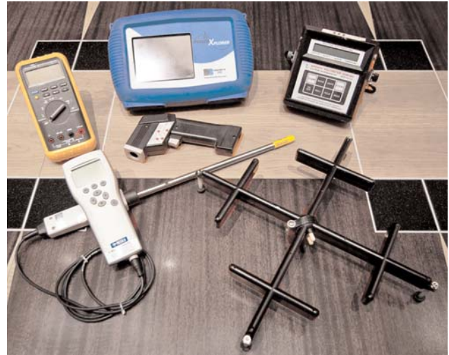
FIGURE 4 Data gathering for commissioning. A variety of tools and sensors are used to measure airflow speed and pressure, component and air temperature, electrical power and voltage. From Top Left—Counter Clockwise: Fluke 87 Multimeter: Used for general measurement of electrical voltage, current, and frequency. Dranetz PowerXplorer: Used to measure and data log very small fluctuations of electrical voltage, current, and frequency. Primarily used when testing data center electrical systems. Shortridge Instruments-AIRDATA Multimeter—ADM-860: Used to measure airflow, velocity, pressure, and temperature. Vaisala Temperature/Humidity Meter: Used to measure data log temperature and humidity. (Center) Raytek Infrared temperature Gun: Used to measure surface temperatures. (Image and descriptions courtesy Michaud Cooley Erickson Engineers.)
