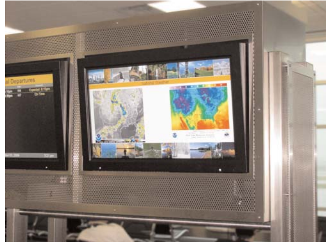
FIGURE 11 Information display. Flight information display retrofit with LCD monitor.
