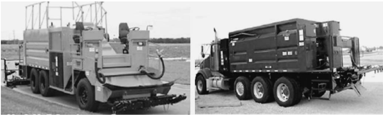
FIGURE 22 Continuous front-loaded self-propelled ( left ) and truck-mounted ( right ) microsurfacing mixing machines ( Courtesy: Bergkamp Inc. 2010 ).
