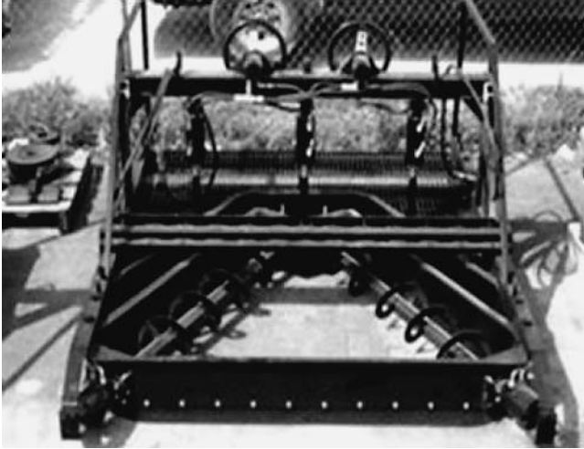
FIGURE 19 Rut box (Courtesy: Bergkamp Inc. 2010).
