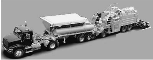
FIGURE 23 Continuous front-loaded self-propelled being resupplied by a mobile support unit (Courtesy: Bergkamp Inc. 2010).
