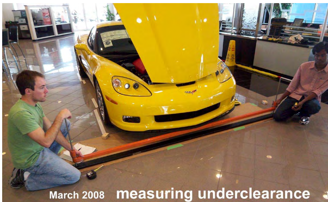
EXHIBIT 4-3 Measuring vehicle ground clearance
