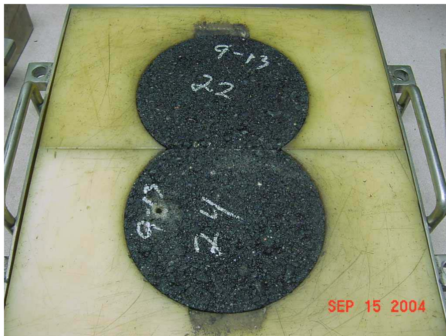
FIGURE 1 Two gyratory pills, 61 mm in height, at a target air voids of 7\% \pm 0.5\% , are arranged to produce a single test specimen.
