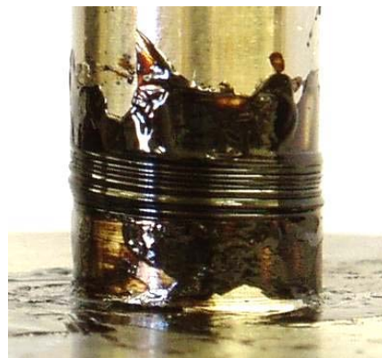
FIGURE 3 Photograph of failed asphalt binder subjected to constant shear rate loading.
