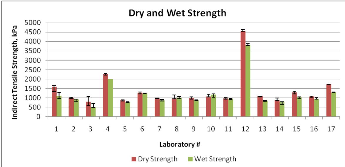
Figure 3-7- Average dry and wet strength values of Marshall compacted sandstone specimens
