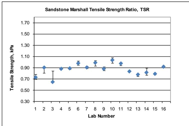
Figure E-2- Error band of indirect tensile strength properties of sandstone gyratory specimens
