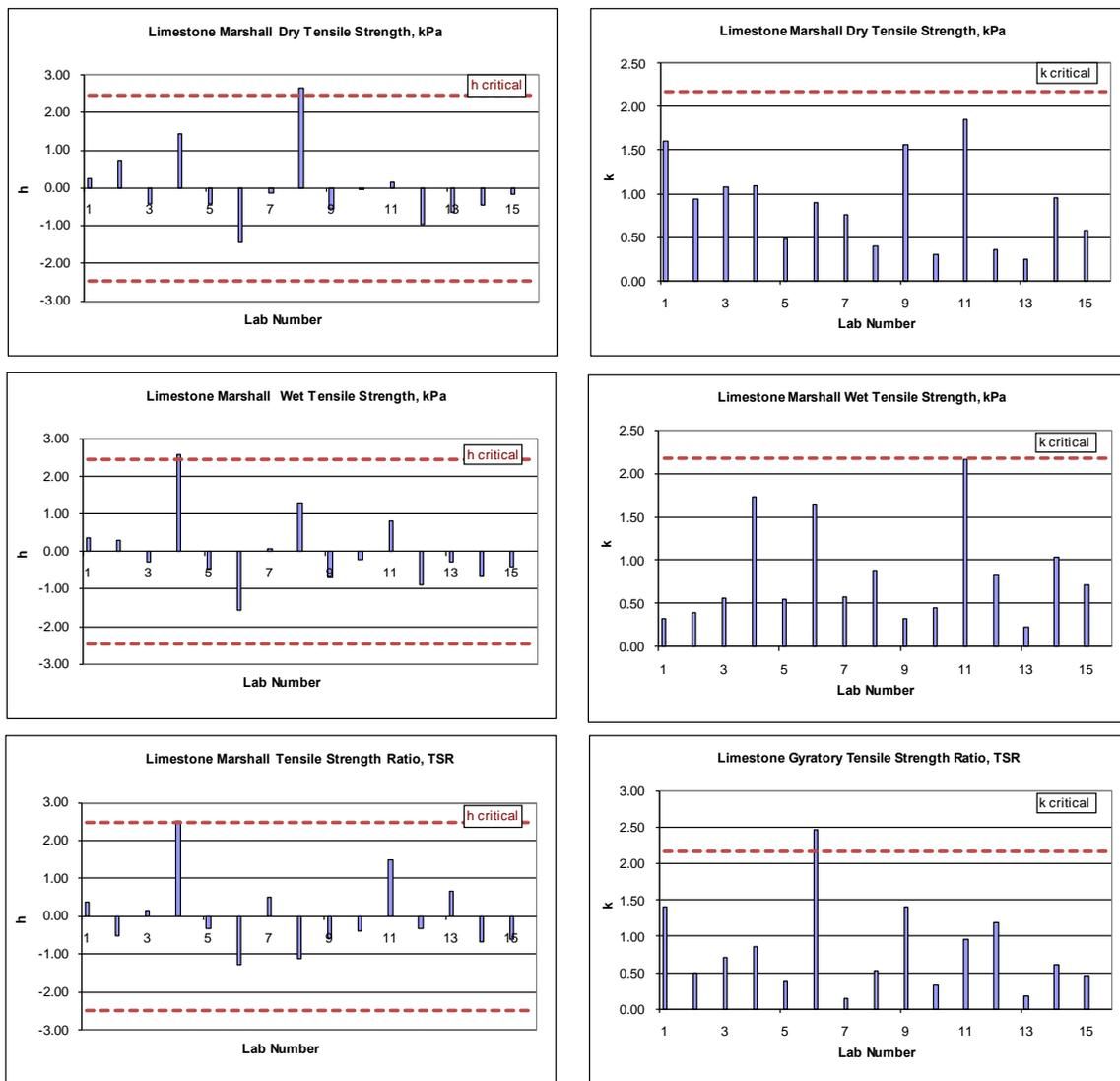
Figure C-1- h and k statistics of indirect tensile strength properties of limestone Marshall specimens
