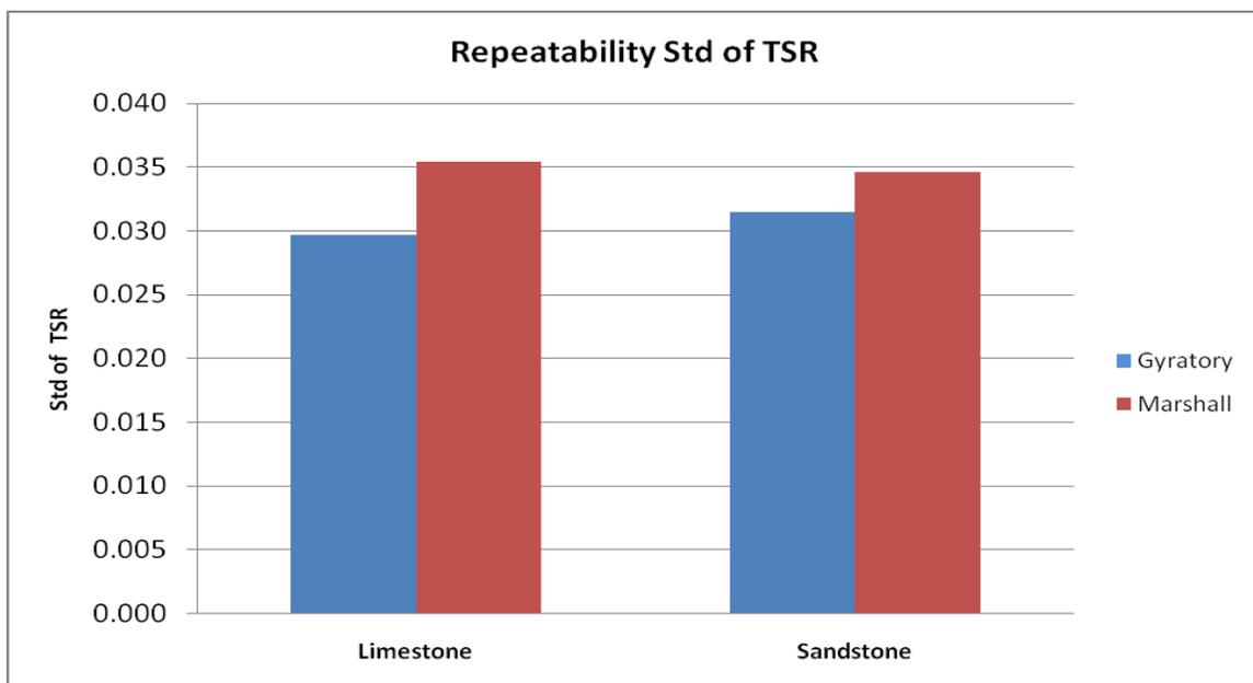
**Figure 3-10- Comparison of the within-laboratory standard deviation of TSR values of gyratory and Marshall compacted limestone and sandstone specimens**
