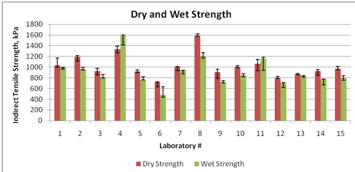
**Figure 3-3- Average dry and wet indirect tensile strength values of Marshall compacted limestone specimens**
