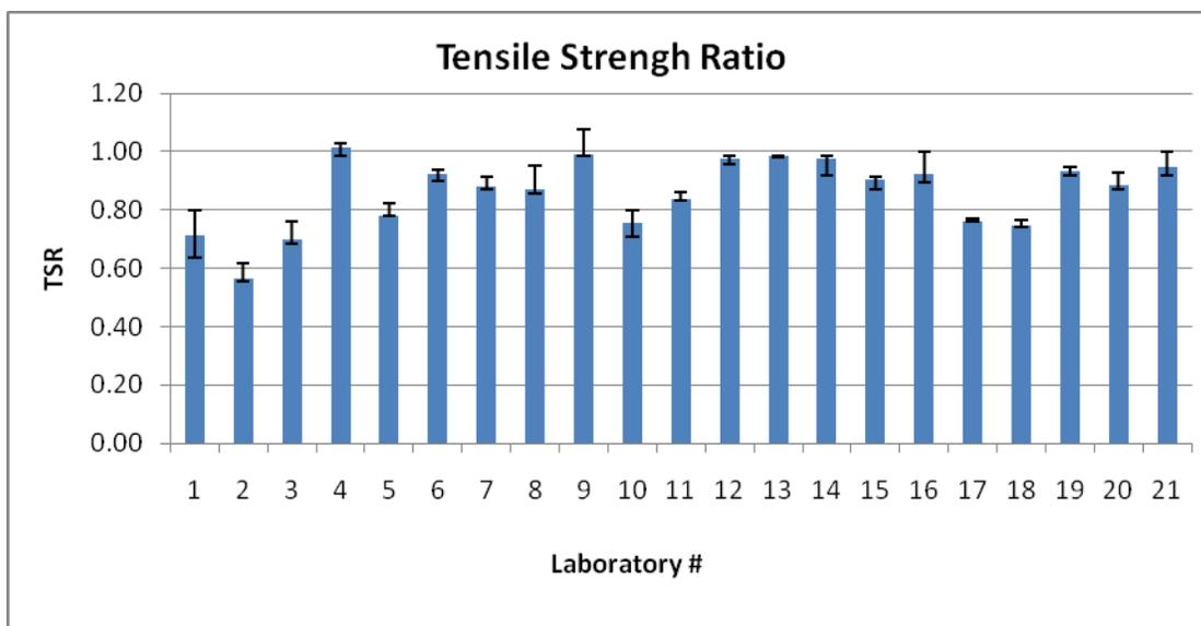
**Figure 3-6- Average TSR values of gyratory compacted sandstone specimens**
