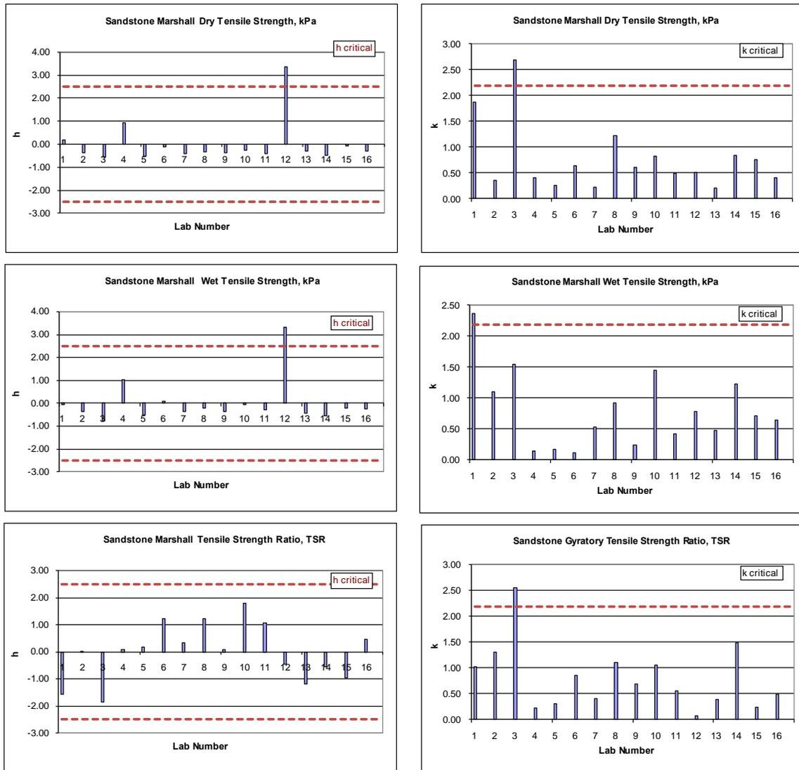
Figure E-1- h and k statistics of indirect tensile strength properties of sandstone Marshall specimens
