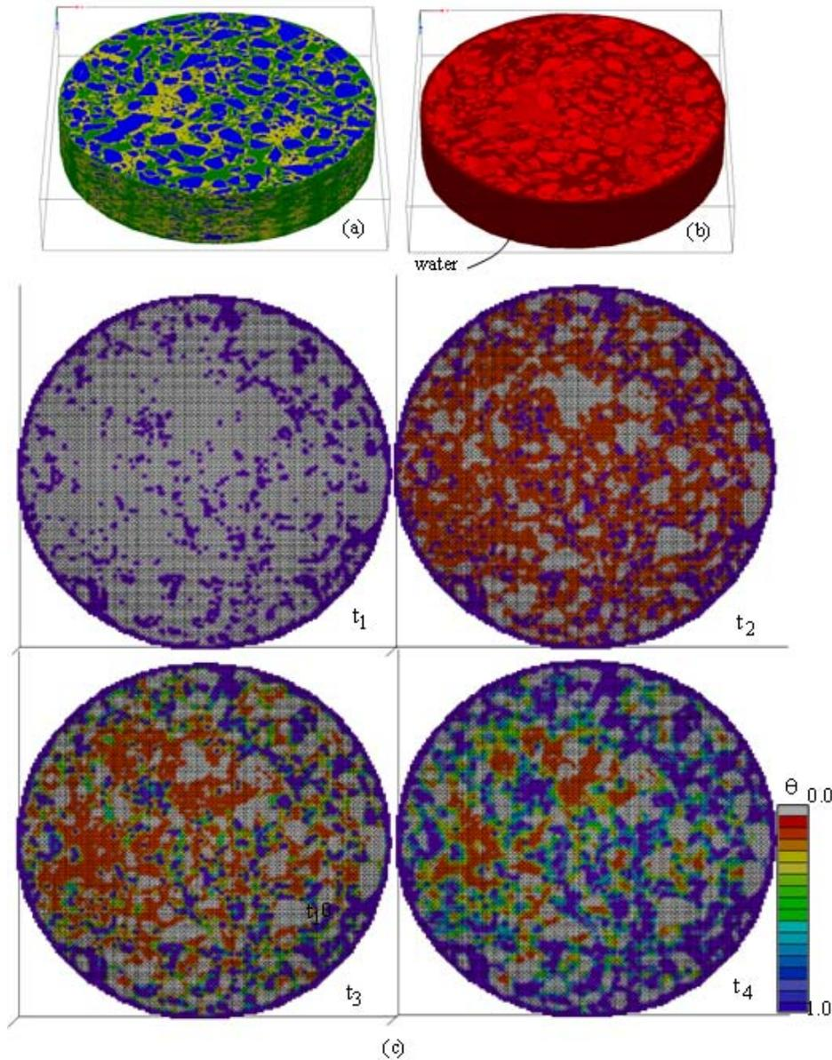
**Figure 4-5- Finite element infiltration in Gyratory compacted limestone (LMS) specimen (a) finite element mesh (b) moisture conditioning (c) moisture infiltration in mid-plane for different conditioning times  $t$ , in which  $\theta$  is the moisture content (or normalized moisture concentration)**
