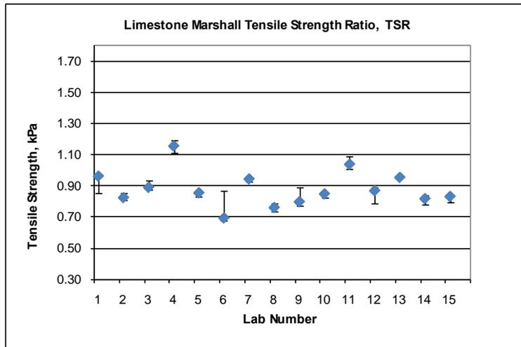
Figure C-2- Error band of indirect tensile strength properties of limestone Marshall specimens
