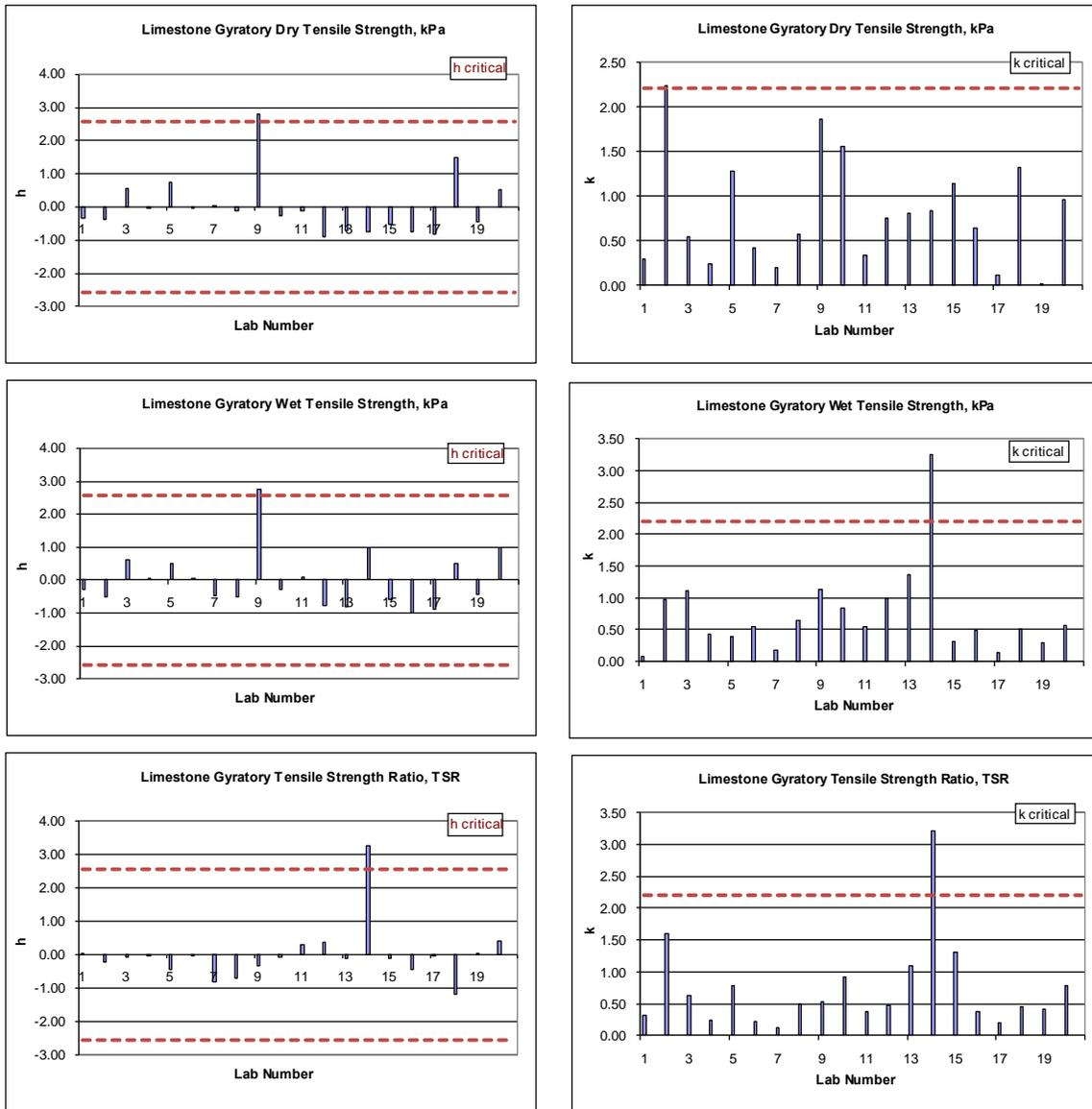
Figure B-1- h and k statistics of indirect tensile strength properties of limestone gyrotary specimens
