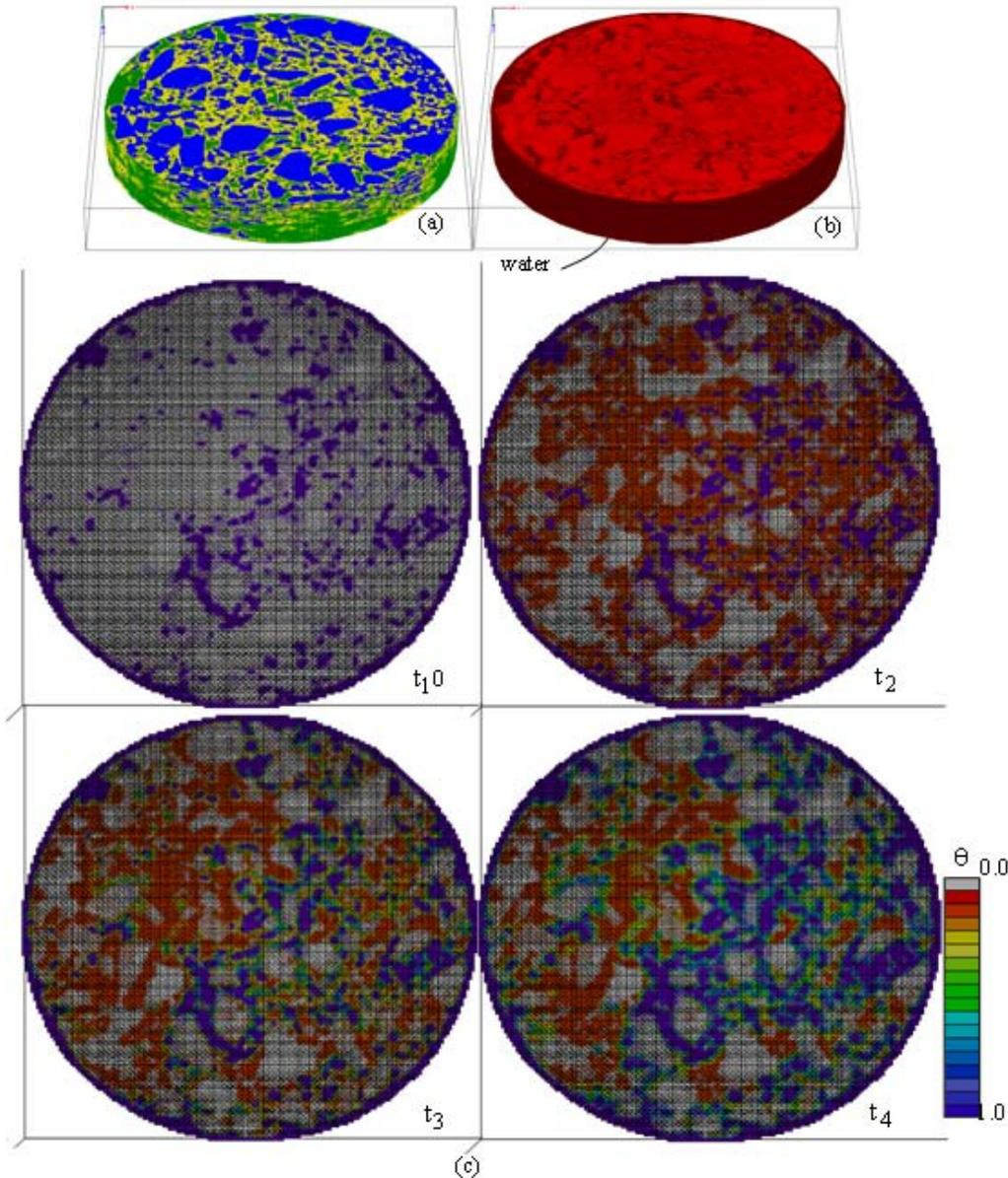
**Figure 4-6- Finite element infiltration in Marshall compacted KST specimen (a) finite element mesh (b) moisture conditioning (c) moisture infiltration in mid-plane for different conditioning times  $t$ , in which  $\theta$  is the moisture content (or normalized moisture concentration)**
