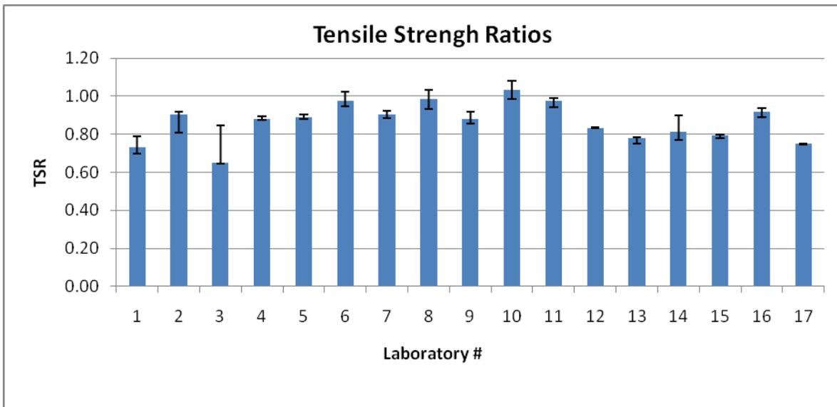
Figure 3-8- Average TSR values of Marshall compacted sandstone mixtures specimens
