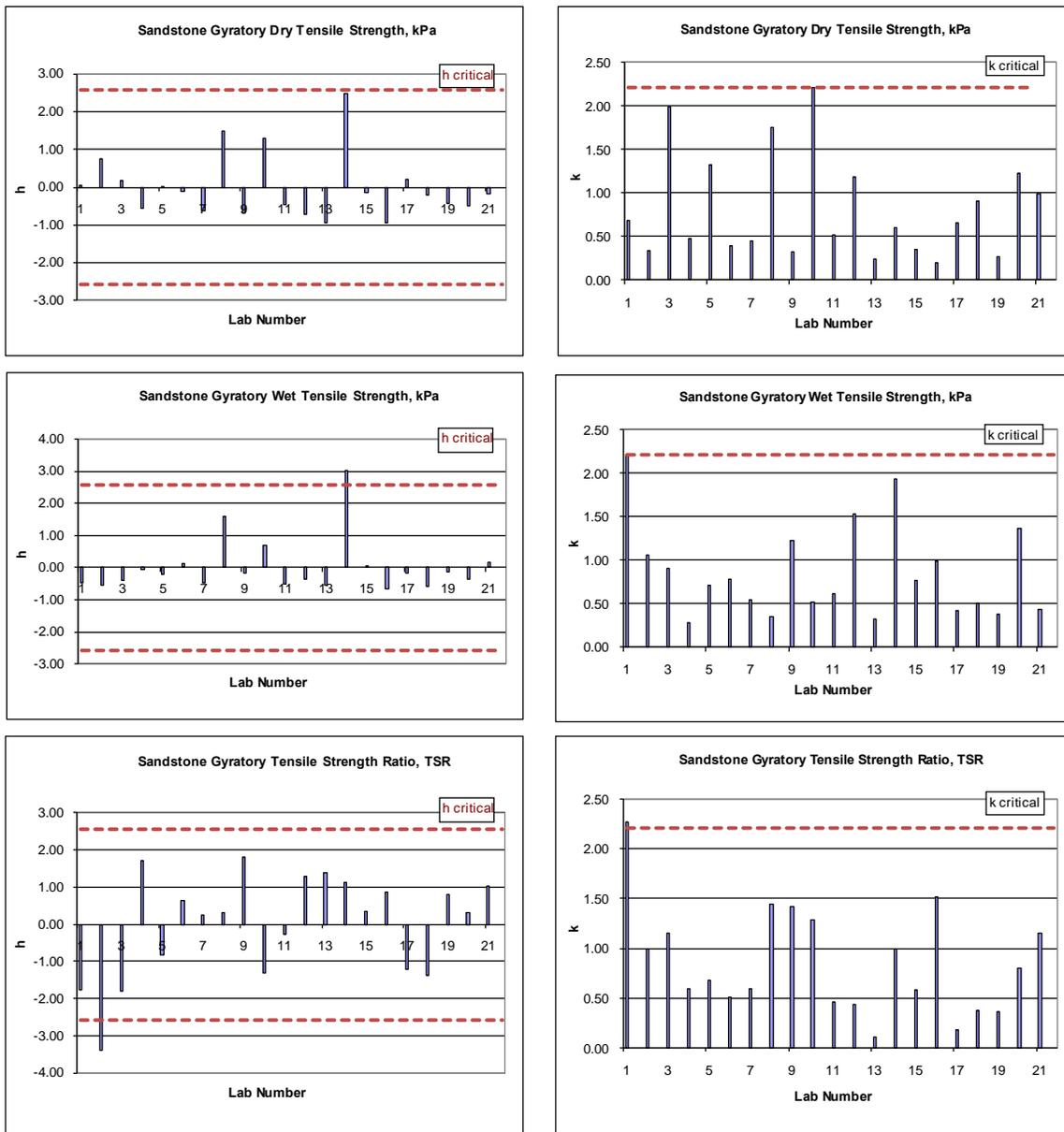
Figure D-1- h and k statistics of indirect tensile strength properties of sandstone gyrotory specimens
