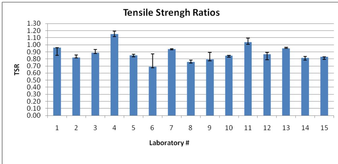
**Figure 3-4- Average TSR values of Marshall compacted limestone specimens**
