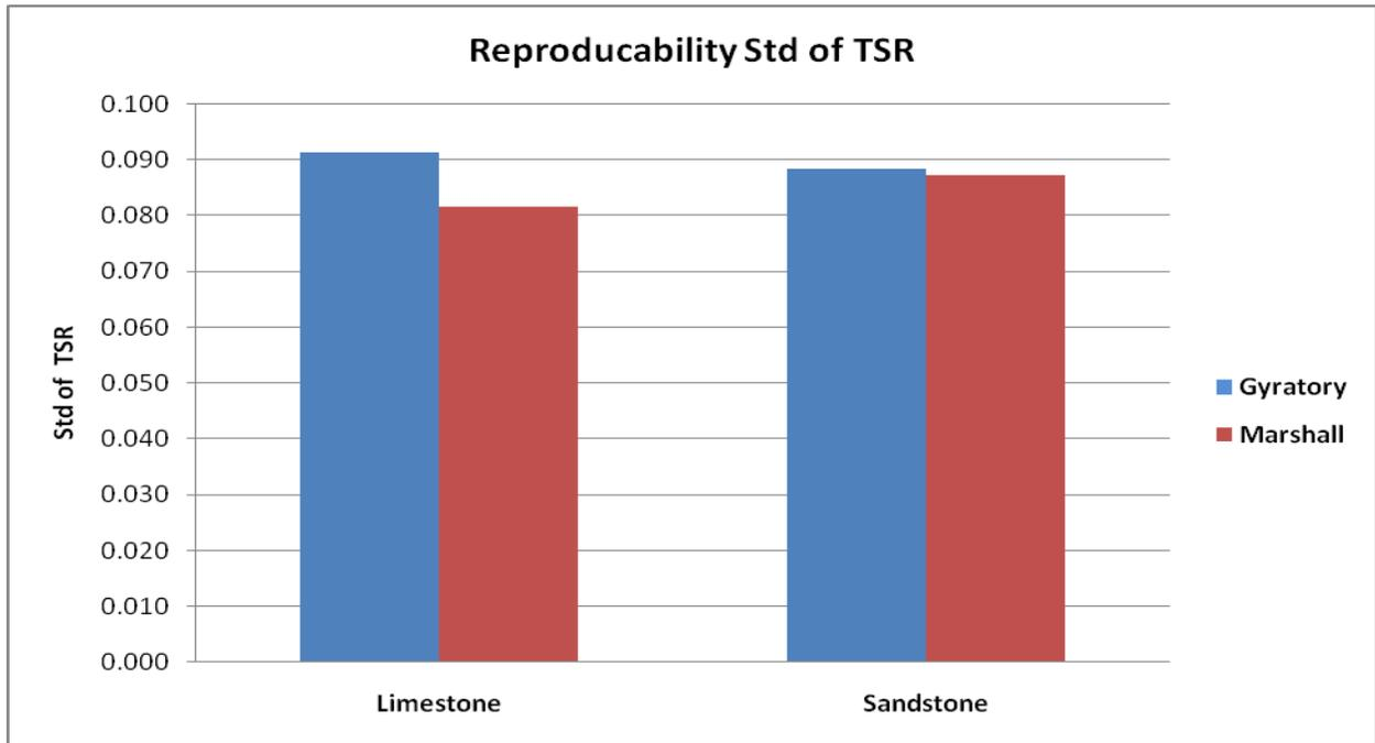
**Figure 3-11- Comparison of the between-laboratory standard deviations of TSR values of gyratory and Marshall compacted limestone and sandstone specimens**
