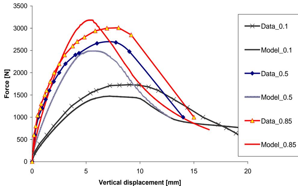
Figure 4-8- Comparison of laboratory indirect tensile test data and CAPA-3D simulation at different loading rates
