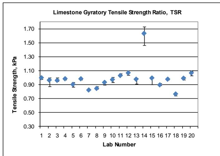
Figure B-2- Error band of indirect tensile strength properties of limestone gyrotory specimens
