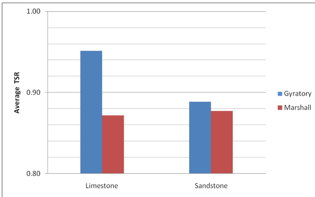
**Figure 3-9- Comparison of the average TSR values of gyratory and Marshall compacted limestone and sandstone specimens**
