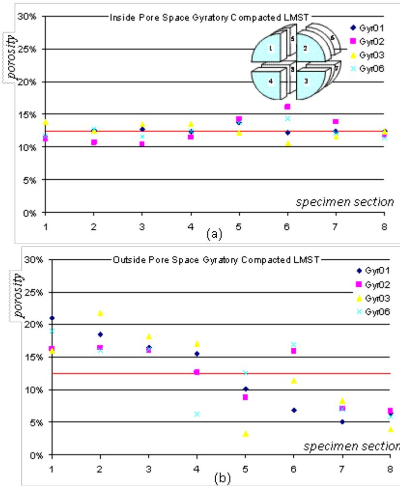
**Figure 4-3- Pore space distribution in gyrotory compacted limestone (LMST) specimens (a) inside porosity (b) outside porosity**
