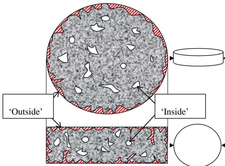
Figure 4-2- Schematic of inside and outside pore-space
