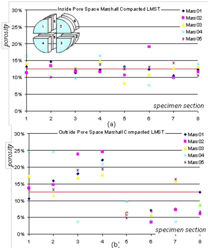
Figure 4-4- Pore space distribution in Marshall compacted limestone (LMST) specimens (a) inside porosity (b) outside porosity
