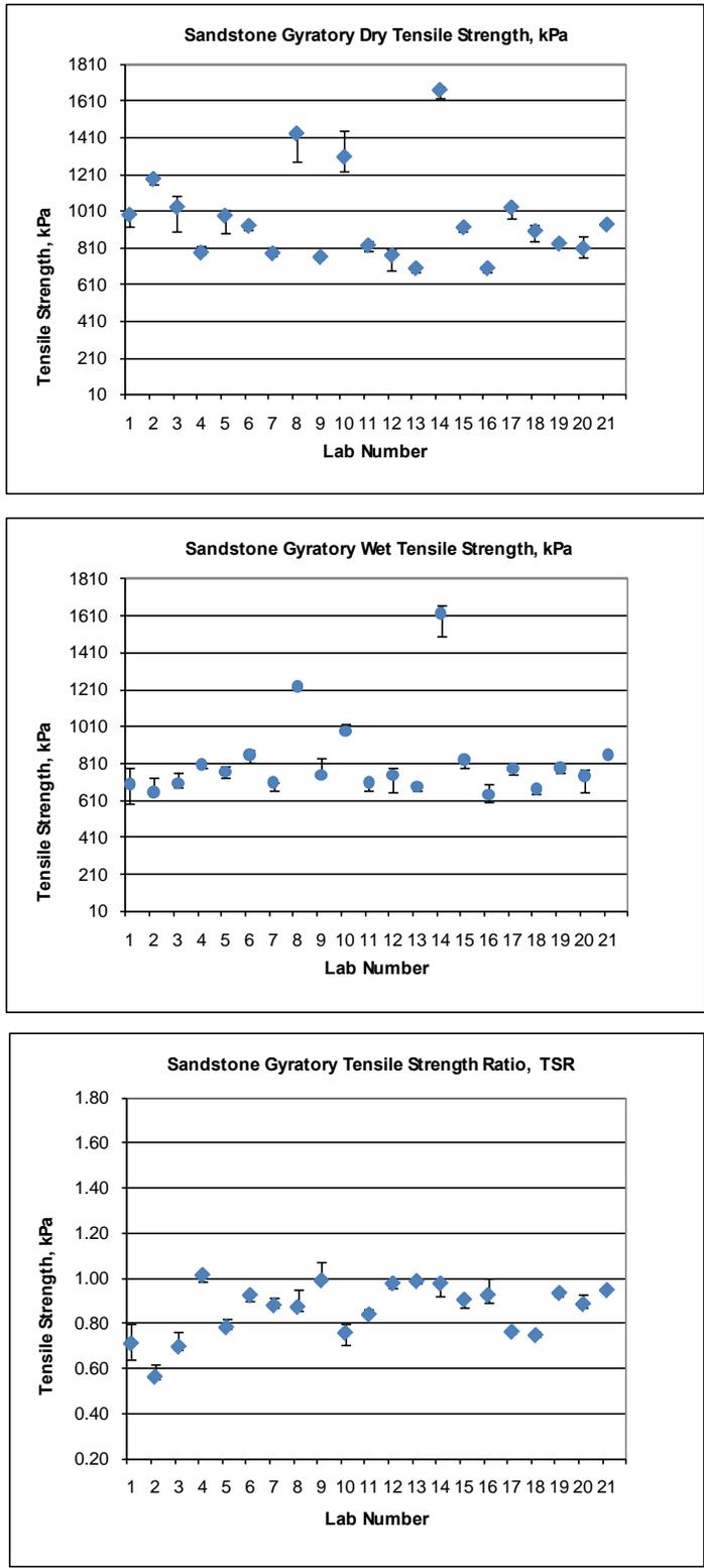
Figure D-2- Error band of indirect tensile strength properties of sandstone gyrotory specimens
