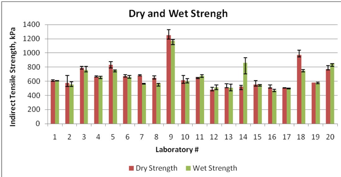
**Figure 3-1- Average dry and wet indirect tensile strength values of gyratory compacted limestone mixtures**
