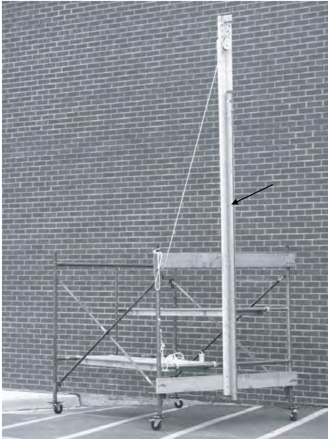
Figure 14. Apparatus to test impact resistance of a falling tup. (The metal guide tube is indicated with an arrow. The casters allow easy positioning of the impactor over the detectable warning system. The mass and tup have been retracted through the guide tube.)
