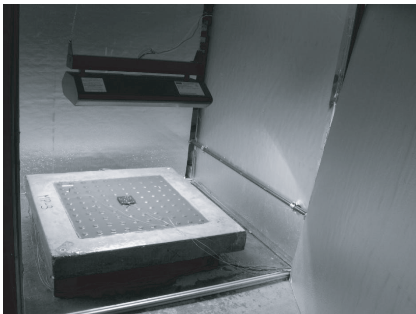
Figure 2. Enclosure and sample under heating (ramp) portion of test cycle.
