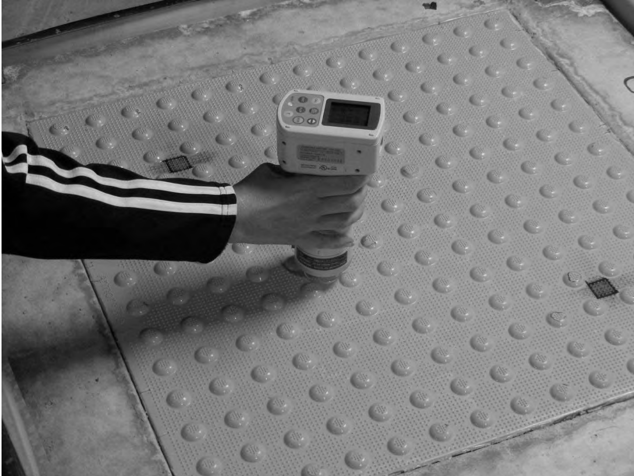
Figure 1-- Measuring the color of the field with a colorimeter with a measuring head of appropriate size to fit between the domes.
