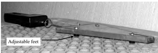
Figure 12. Evaluating slip by the slipmeter (note that the adjustable Neolite feet are centered on the tops of the domes).
