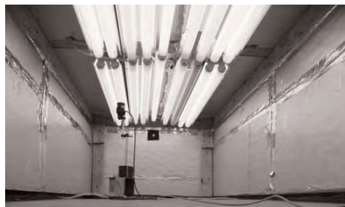
Figure 7. Interior of the UV light exposure enclosure.
