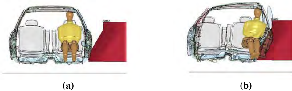
FIGURE 16 Vehicle and SID response at the time of peak injury: (a) initial position and (b) calculated response.
