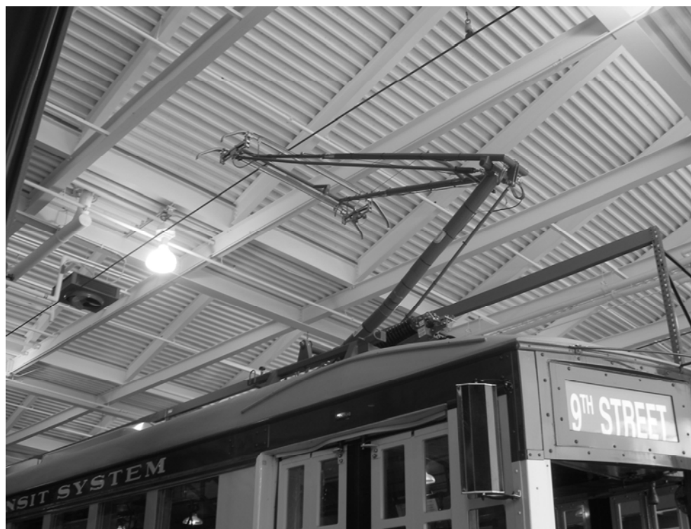
FIGURE 2 Pantographs were installed on Charlotte's replica trolleys to enable them to share track with modern LRVs.
