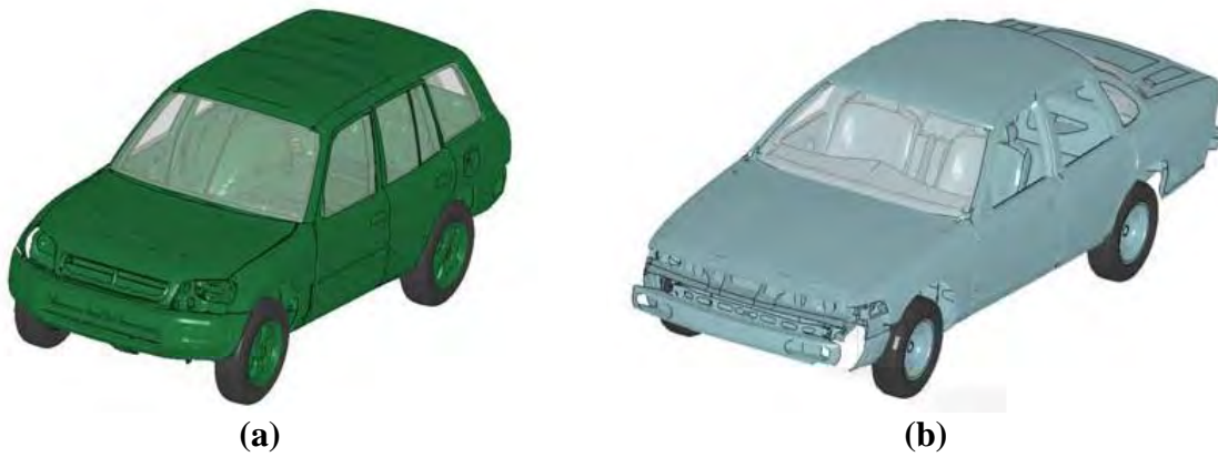
FIGURE 12 Finite element models for the additional highway vehicles used in the crash analyses: (a) HV 3, Toyota RAV4; and (b) HV 4, Ford Crown Victoria.
