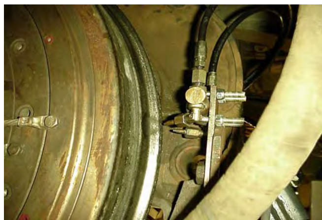
FIGURE 13 Onboard lubricator: flange lubricator on LRV117.
