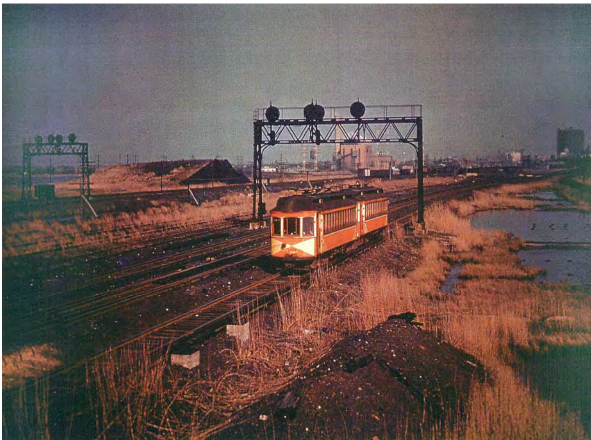
FIGURE 1 A Shore Fast Line Interurban passes under a PRR position light signal on its way into Atlantic City. Once in Atlantic City, this train will leave the main track and operate over streetcar tracks to the boardwalk. An example of simple technology and sound OD in the days before we needed to rely on Maglevs, monorails, and other advanced concepts to get to the boardwalk.
