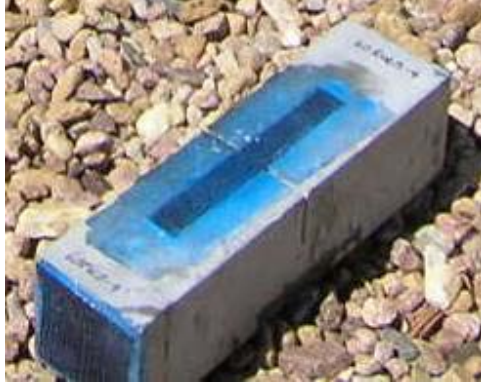
Figure 21. Completed specimen with end patch
