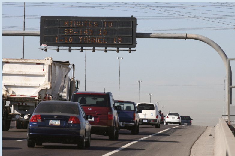
Speed management techniques, such as this dynamic message sign in Phoenix, Arizona, can help reduce vehicle emissions.
