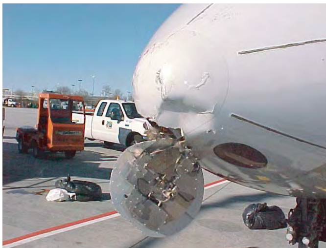
On approach to an eastern U.S. airport, this CRJ with 35 people on board sustained a goose strike to the radome, at 250 knots. There was major damage to the radome and electronic components. (Photo courtesy FAA)
