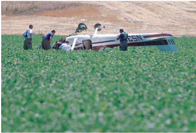
This Cessna 150 crash-landed in a tomato field and was damaged beyond repair after a hawk shattered the windshield during approach to a western U.S. airport on July 20, 2007. (Photo courtesy USDA)
