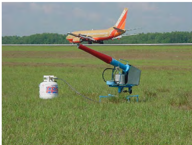
Propane cannons will quickly lose their effectiveness if used constantly without lethal reinforcement. (Photo J. Metcalf, GOAA)
