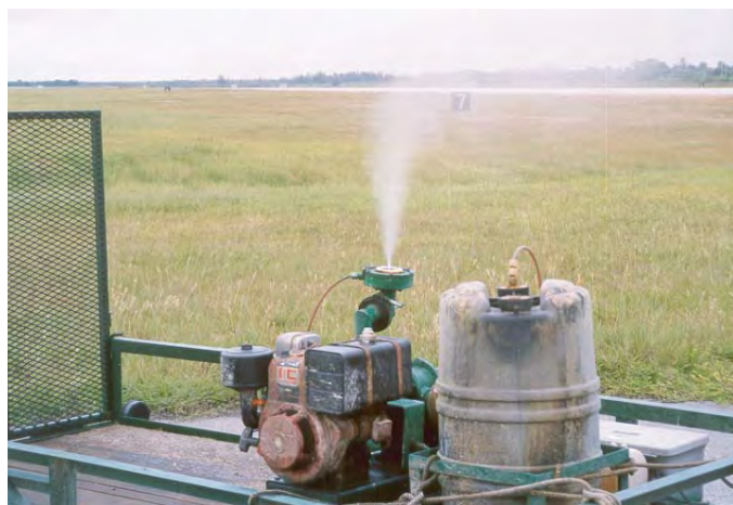
A methyl anthranilate formulation is available for use in fogging machines (thermal or mechanical) to disperse birds from hangars, lawns, and other areas. (Photo courtesy USDA)
