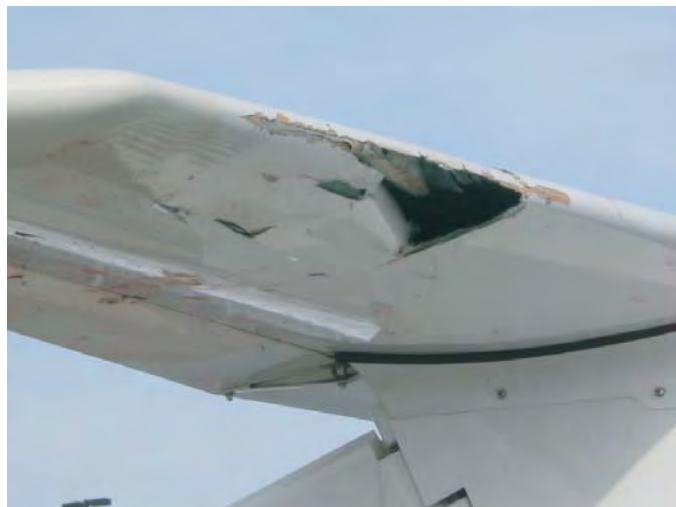
Whenever possible, photograph all bird strike damage. This Diamond 20 struck a tundra swan at 2,000 ft AGL, 120 kts, and sustained over $32,000 in damage. (Photo courtesy of FAA)
