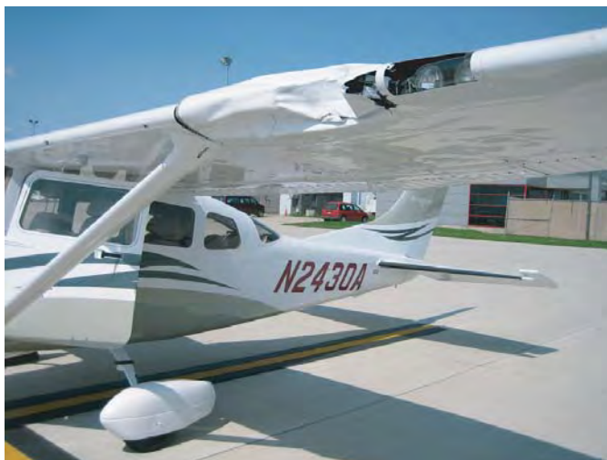
This Cessna aircraft, with only 80 hours of flight time, struck a large bird over a lake several miles from a midwestern airport. (Photo M. Mullen)
