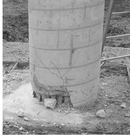
Figure 55. Small standoff blast damage: Column 2A2.
