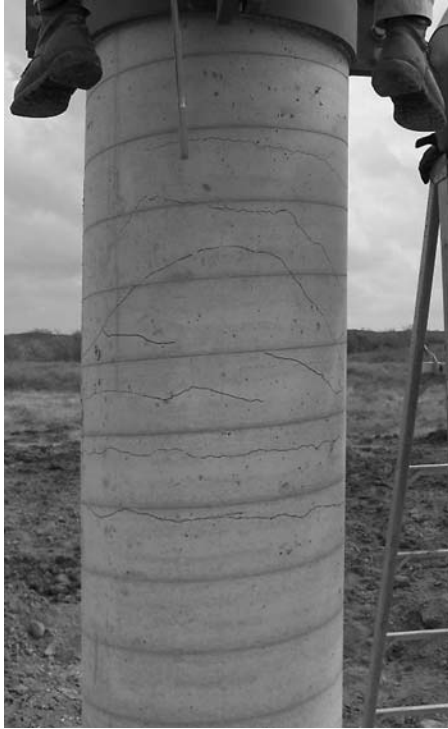
Figure 55. Small standoff blast damage: Column 2A2.
