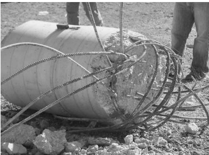
Figure 61. Local damage Test 1: Column 2A2.
