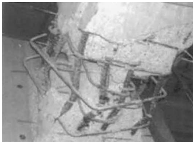
Figure 15. Opening of discrete ties (Bae and Bayrak, 2008).
