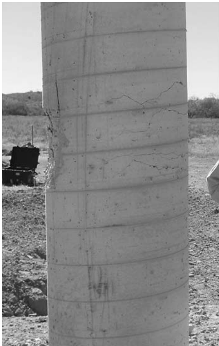
Figure 58. Small standoff blast damage: Column 2-Blast.
