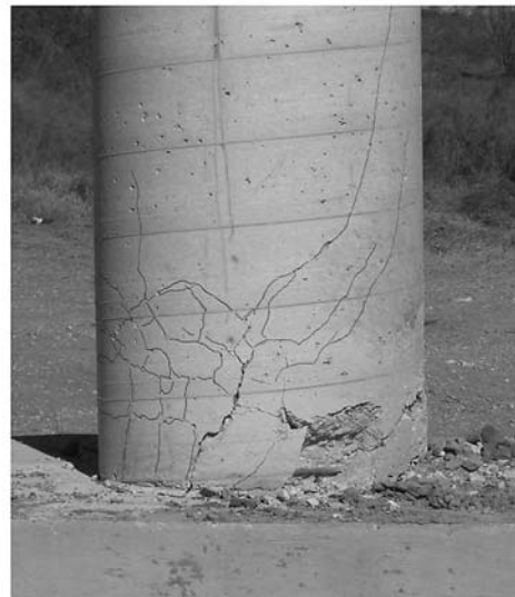
Figure 58. Small standoff blast damage: Column 2-Blast.
