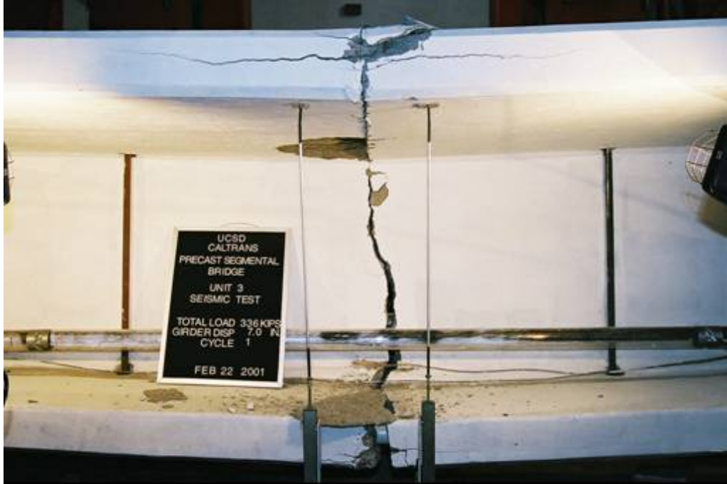
Figure 4. Test unit with 100% external tendons (Photo by Sami Megally)
