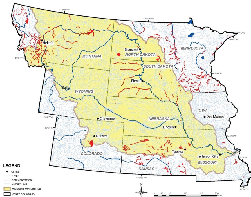
FIGURE 6-5 Missouri River basin streams that are impaired by excess sediments and for which TMDLs have been developed. SOURCE: USEPA, 2010b.
