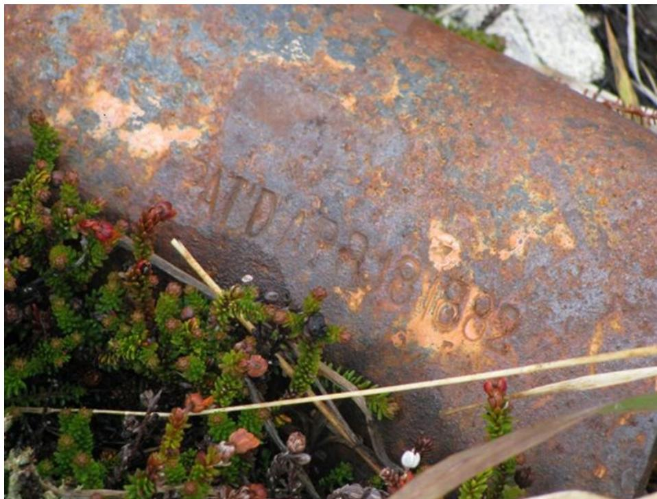
FIGURE 3.6 A ferrous based alloy exposed to the environment since 1882 (note the date on the part). With a cold and dry environment the corrosion process is very slow. SOURCE: University of Virginia Center for Electrochemical Science and Engineering, courtesy of John R. Scully and UVA MSE 3080 class participant.
