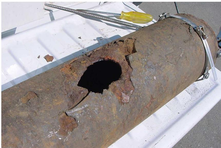
FIGURE 1.3.2 A failed cast iron pipe. Courtesy of Mark Lewis, East Bay Municipal Utility District.
