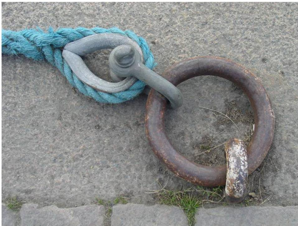
FIGURE 1.1 A mooring ring, shackle, and thimble with rope illustrate three different techniques for combatting the effects of materials degradation. Originally, the ring and eye bolt were painted, the shackle and thimble were galvanized (zinc coated), and the mooring line was made of nylon. Courtesy of Erik Svedberg.
