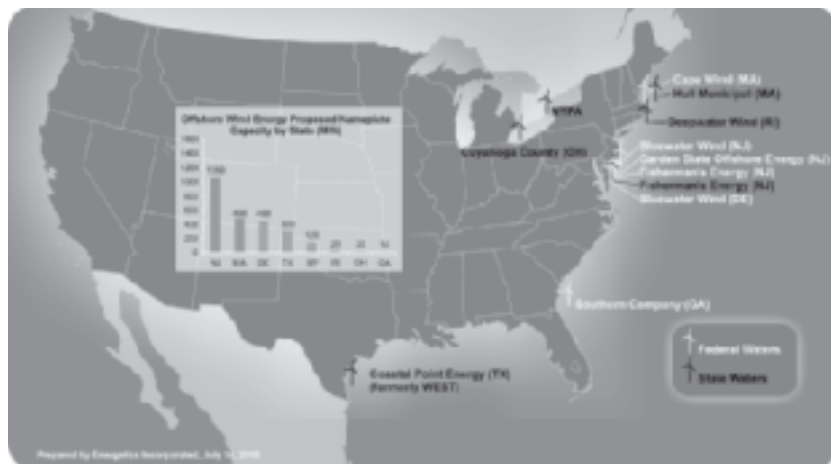
FIGURE 2-11 Proposed U.S. offshore wind projects and capacity showing projects with significant progress. (SOURCE: Musial and Ram 2010.)
