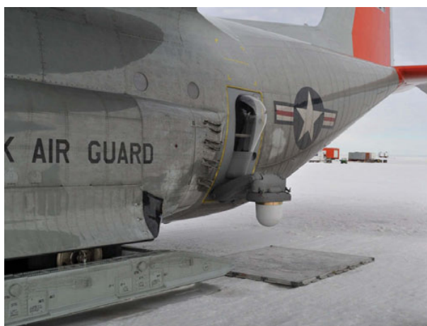
FIGURE C.4 Hercules turboprop aircraft modified for Antarctica. Current design is LC-130 with modifications that allow LIDAR and RADAR observations of continental ice characteristics and thickness. SOURCE: E. Dunlea.
