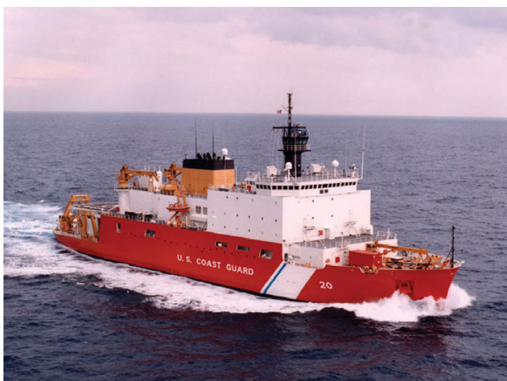
FIGURE D.1 Examples of the attributes of a variety of icebreakers: (a) Russian (Lukoil, Ltd.) icebreaker Varandey , service ship, length 100 m, maximum power 16.8 MW from two azimuthing electric pods; (b) U.S. Coast Guard icebreaker Healy is designed for heavy ice and polar research missions of NSF, length 130 m and maximum power 22 MW; (c) NSF (University of Alaska, Fairbanks) owned Sikuliaq , research light icebreaker (PC6-7) to be launched in 2013; (d) USCG Polar Sea/Star, length 122 m, maximum power 45 MW (60,000 hp); in repair to 2013. SOURCES: (a) Chenghui, 2011, (c) Edgar, 2011, both reprinted with the permission of the Society of Naval Architects and Marine Engineers (SNAME); (b) and (d) U.S. Coast Guard.
