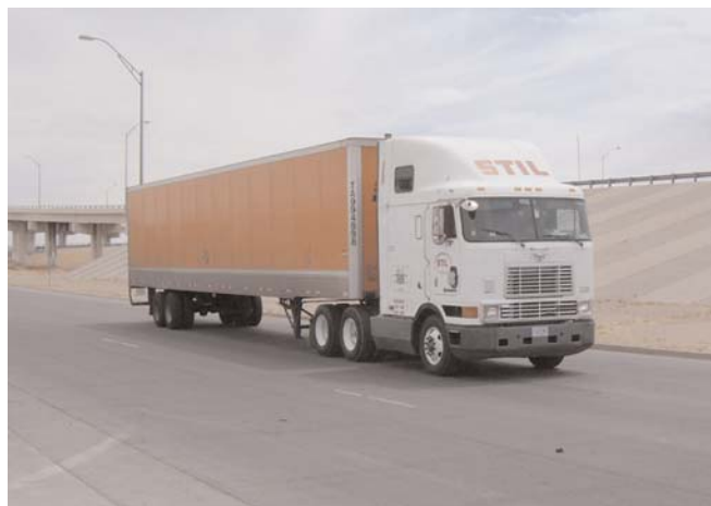
Figure 4 T3-S2 vehicle used in Mexico and operating in Texas.
