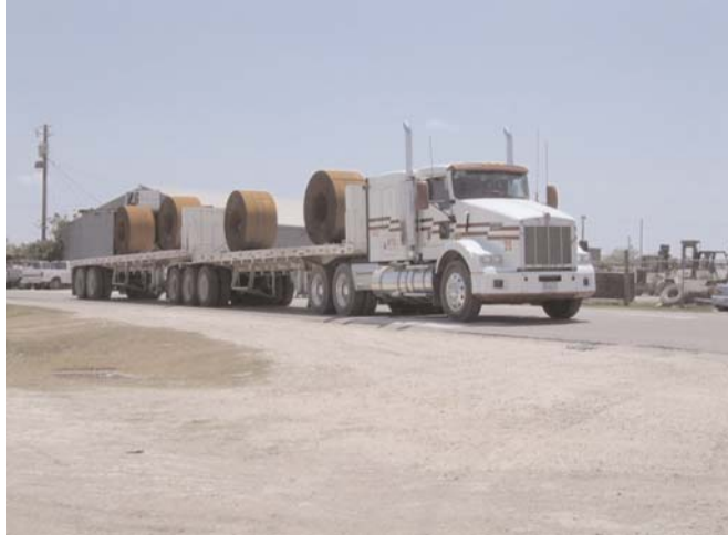
Figure 6 T3-S3-S2 LCV used in Mexico.
