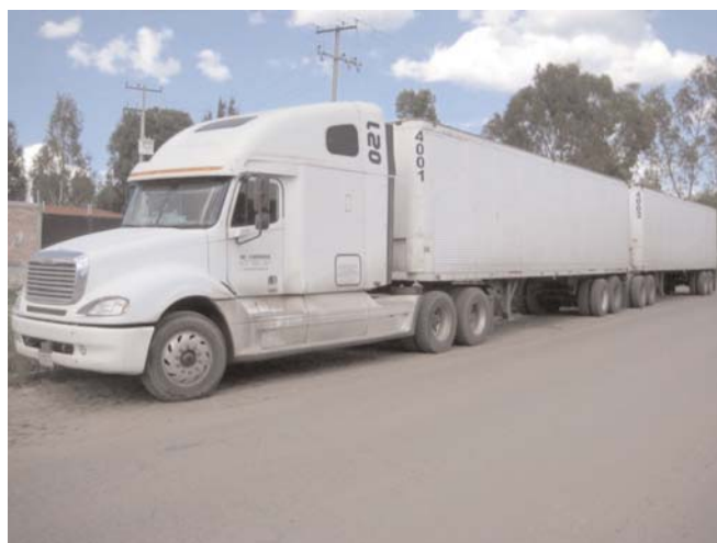
Figure 5 T3-S2-R4 LCV used in Mexico.
