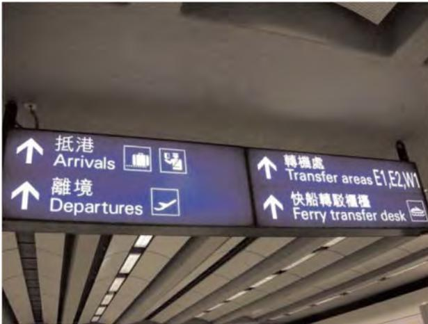
**Figure 6.63a.** Internal illumination of the entire face.
