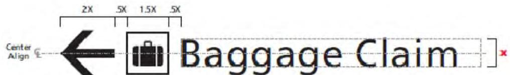
Figure 6.39. Spacing example of relationship between an arrow, symbol, and message.
