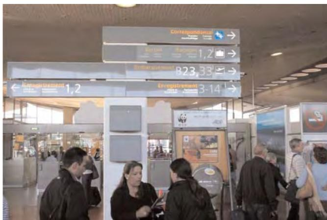
**Figure 6.23.** Example of information overload with a combination of format, number of signs, and amount of information.
