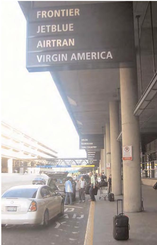
**Figure 5.6. Example of airline identifier signs with multiple carriers per sign (SeaTac International Airport).**
