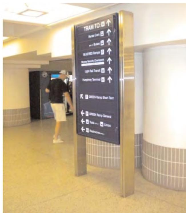
Figure 6.73. In the Minneapolis International Airport Sign System by Apple Design, multiple changes in ceiling height require different font heights to be used.
