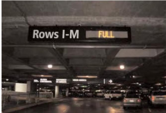
*Figure 4.17. Once inside the garage additional signs indicate the availability of parking within a particular area. In this case, areas are defined by groups of parking aisles. (SEA)*
