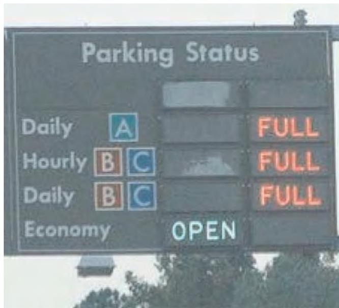
**Figure 4.15.** Roadway sign providing information as to the availability of parking in each parking facility. The information is provided prior to the decision point where driver must travel (Reagan National Airport).
