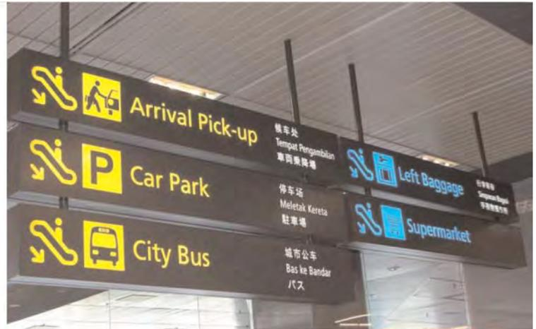
**Figure 6.63b.** Internal illumination of text only.
