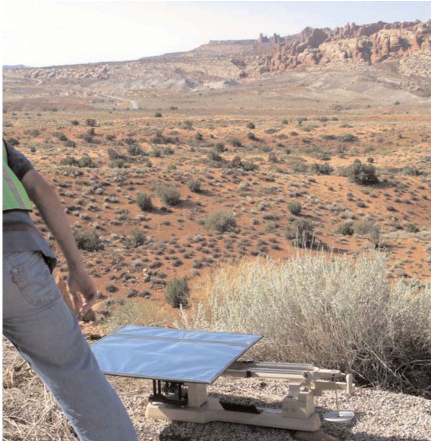
Figure 5. Moisture test pads prior to spraying/chipping.
