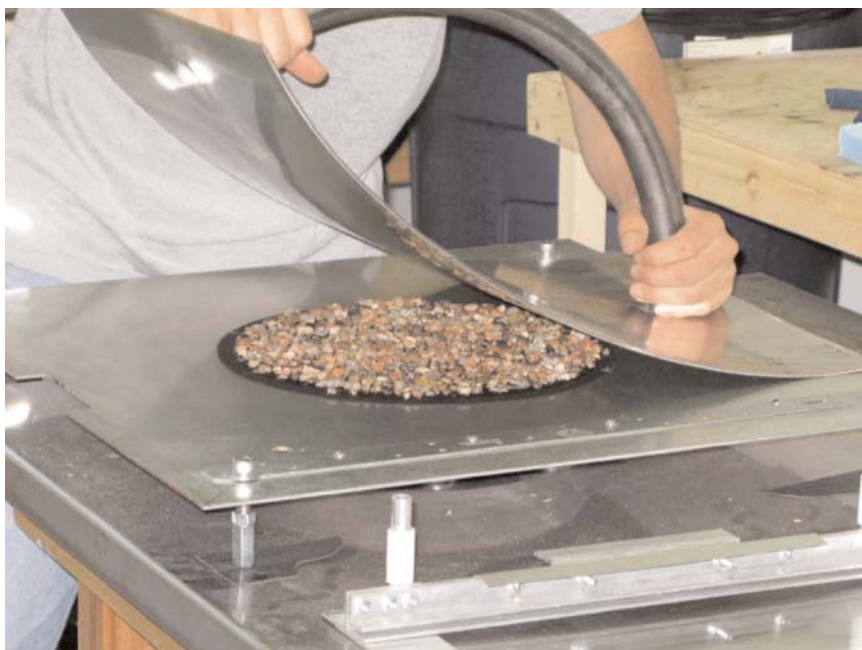
Figure 3. Compactor setting aggregates on test pad.
