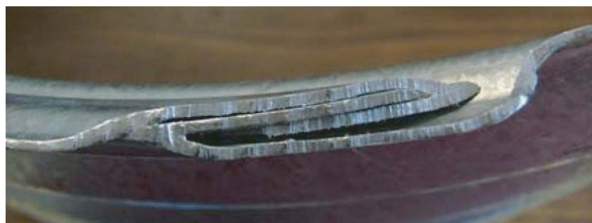
(b) Close-up of Lock Seam
