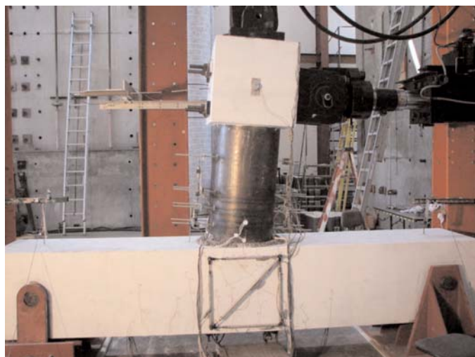
Figure 2.78. Specimen response at 6% drift—HYB3.
