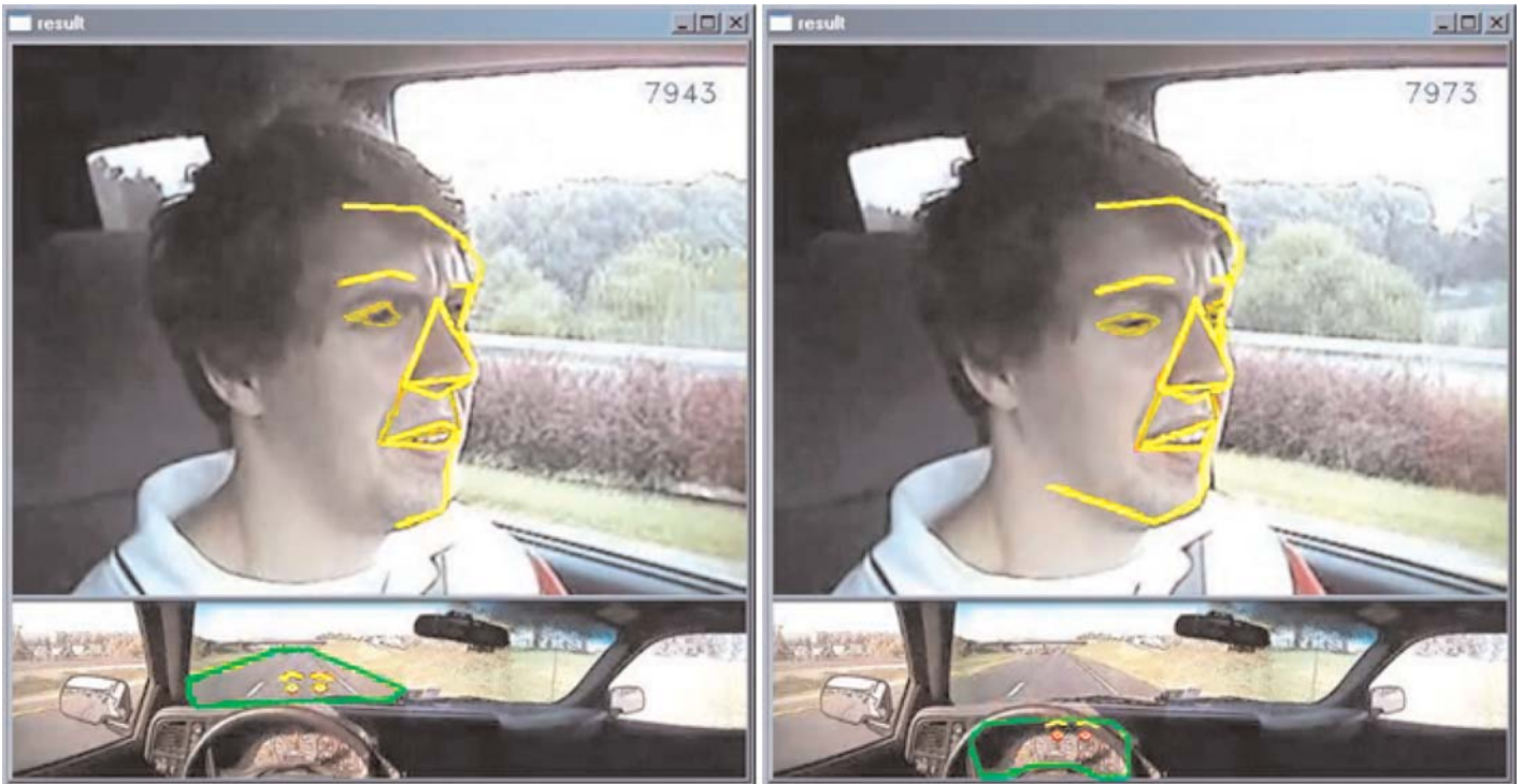
Figure 3.7. VTTI Mask Head Tracker: Calibrated eyes forward (left); calibrated eyes on speedometer (right).
