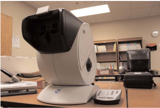
Figure 3.1. Optec 6500P all-in-one vision test apparatus.
