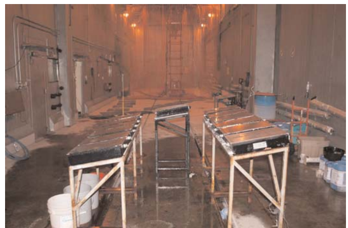
Figure 17. Set-up for leading edge thermal equivalent boxes on test stands at NRC climatic engineering facility.
