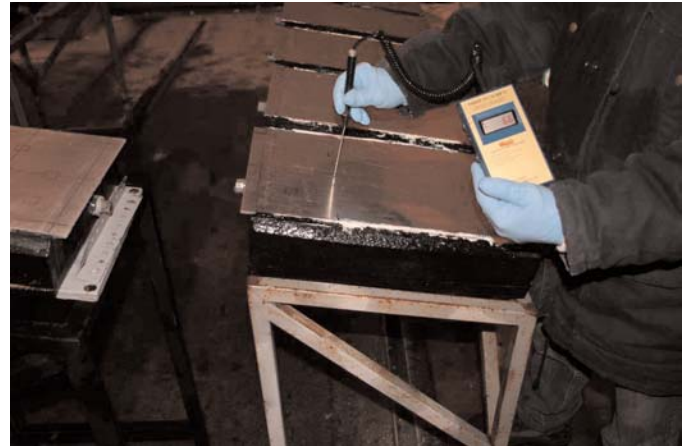
Figure 23. Surface temperature measurements taken from 6-inch line on test plate surface.
