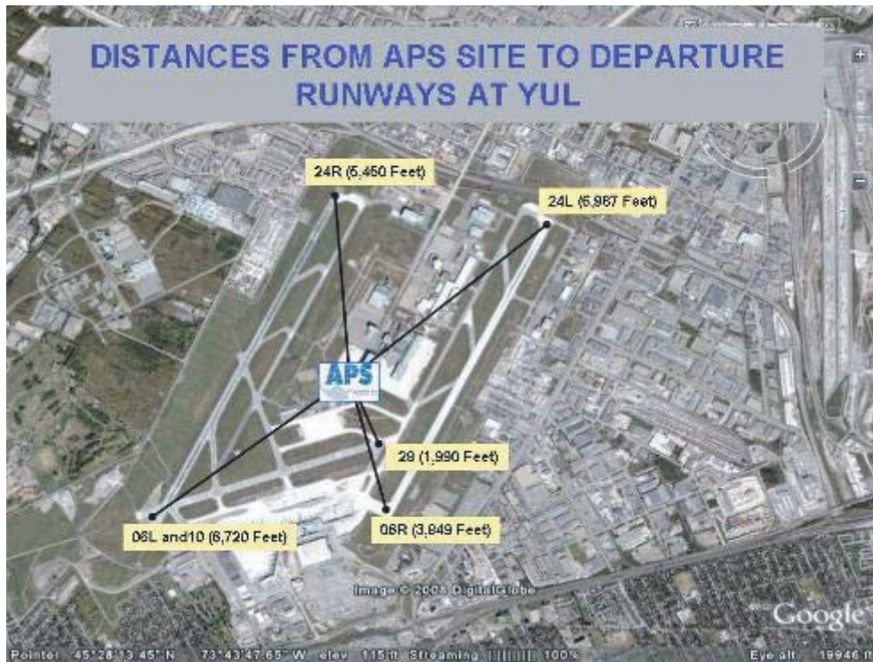
Figure 9. Distances from APS test site to departure runways at Montreal Trudeau International Airport (YUL).
