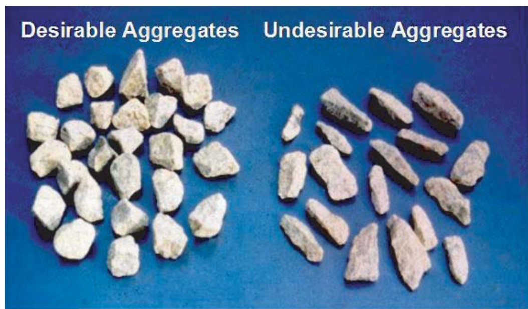
Figure 10-2. Illustration of desirable aggregate shape and angularity.
