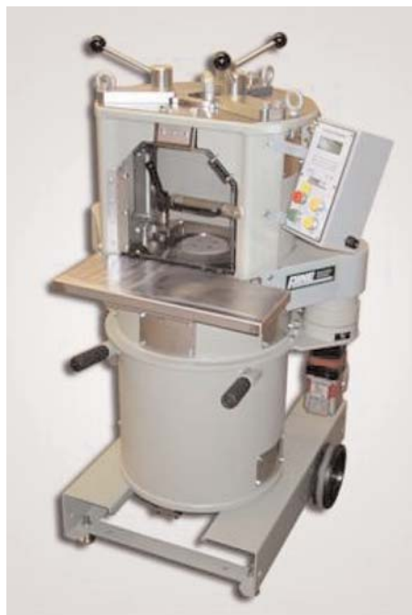
Figure 2-8. Superpave gyratory compactor (Courtesy of Pine Equipment Company).
