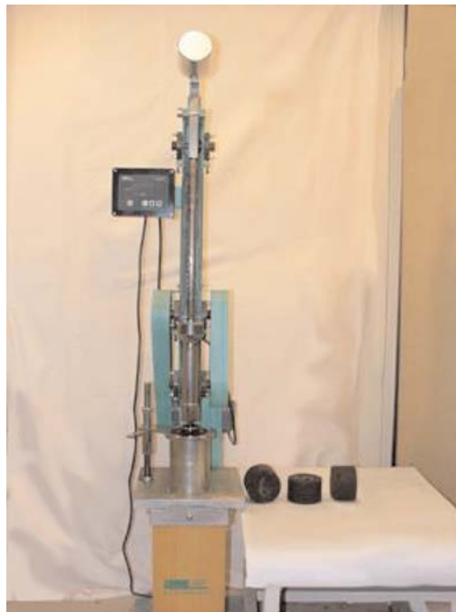
Figure 2-7. Marshall compactor and laboratory specimens for use in the Marshall mix design method.
