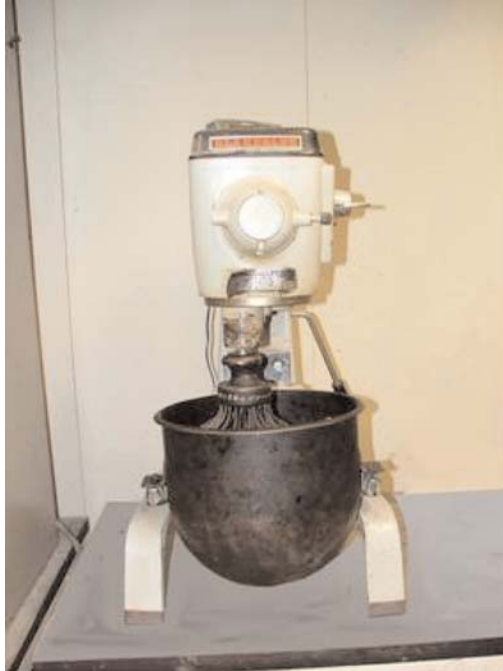
Figure 8-8. Typical mixer used in preparing HMA specimens in the laboratory.
