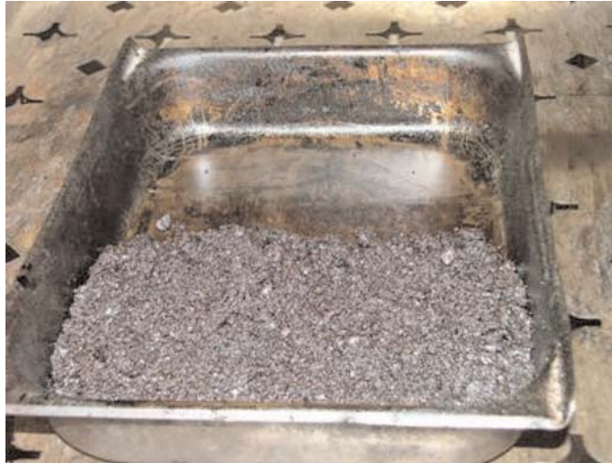
Figure 8-9. Short-term oven conditioning of HMA mixture in the laboratory.
