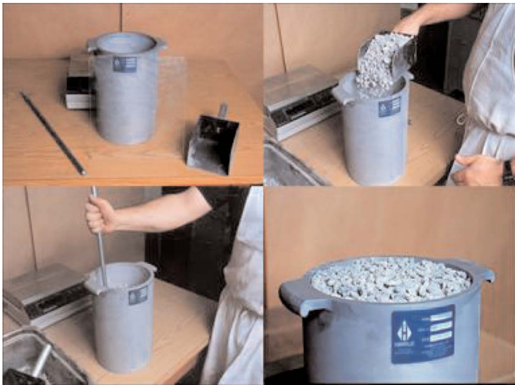
Figure 10-5. Method of determining VCA in dry-rodded condition.
