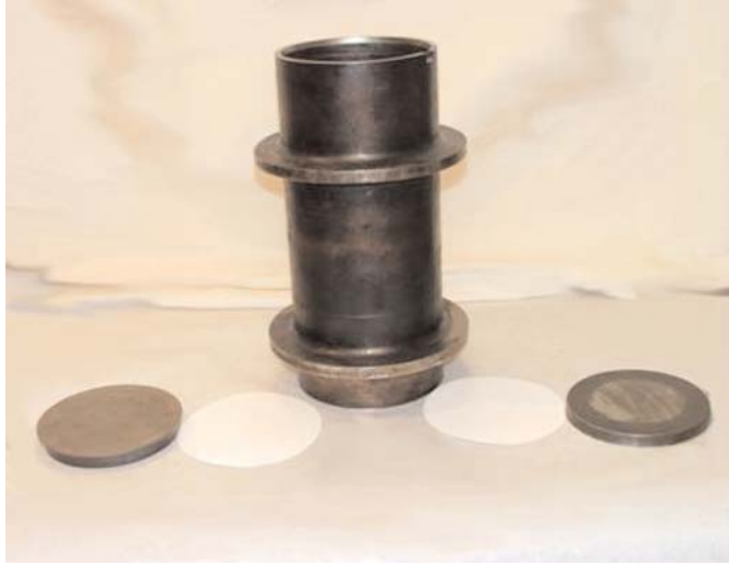
Figure 8-10. Mold, top and base plates, and paper disks used in compacting specimens with the superpave gyratory compactor.
