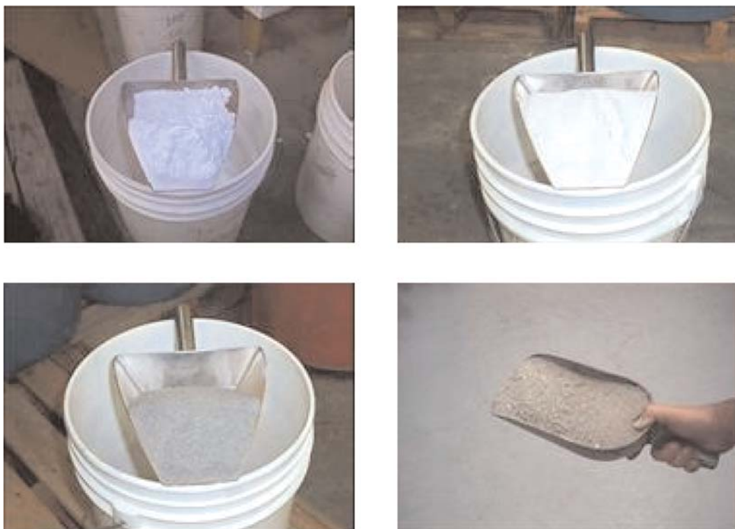
Figure 10-3. Typical mineral fillers used in GGHMA.
