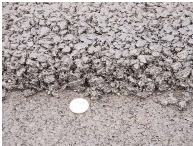
Figure 2-6. SMA surface course on dense-graded HMA base.
