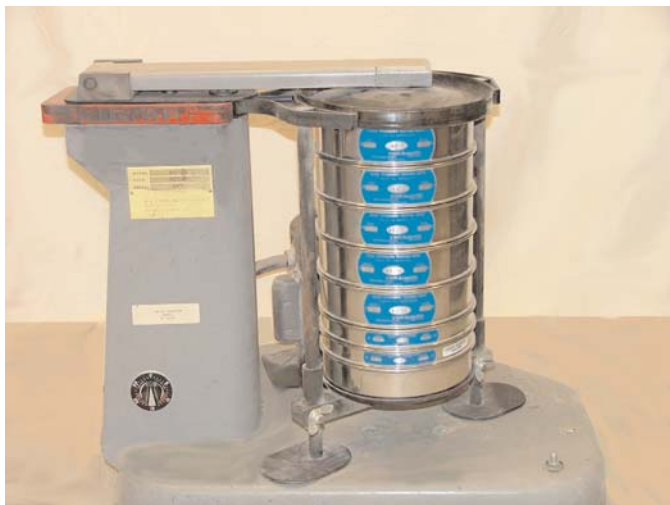
Figure 4-2. Stack of sieves for fine aggregate assembled in a mechanical sieve shaker.
