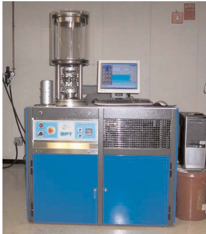
Figure 6-1. Photograph of a simple performance test system.
