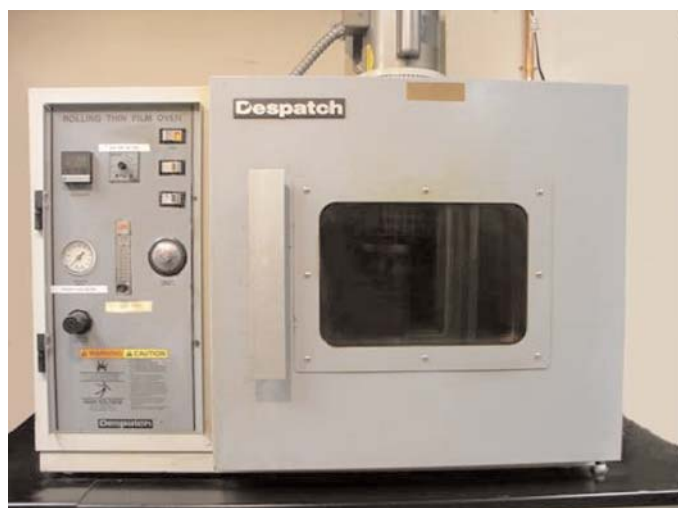
Figure 3-4. RTFOT aging oven.
