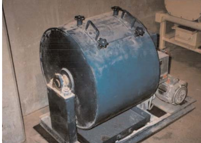
Figure 4-11. Los Angeles abrasion drum.
