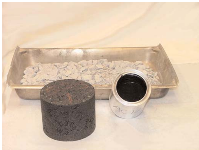
Figure 2-1. A compacted HMA laboratory specimen and the aggregate and asphalt used to prepare it.
