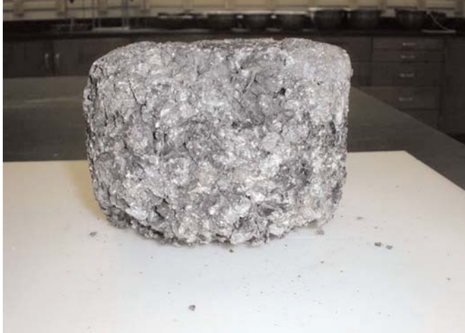
Figure 11-5. Illustration of sample after Cantabro Abrasion test.
