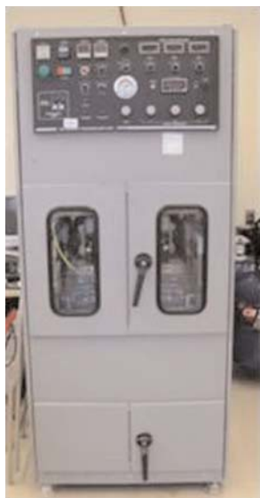
Figure 6-5. Photograph of the asphalt pavement analyzer.
