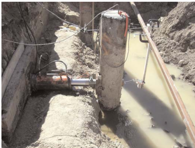
Figure 3-8. Photograph of lateral load test on single pipe pile.
