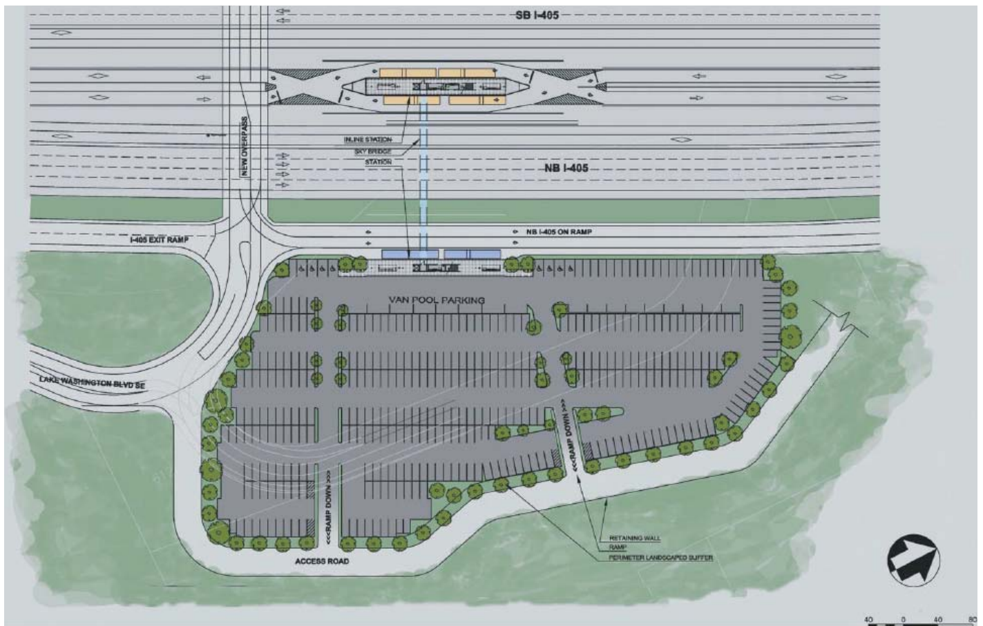
Figure 5-4. Conceptual in-median station and park-and-ride—plan view.
