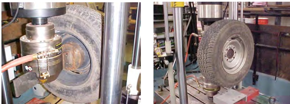
Figure 18. Steel hub and fixture used in the compression test.
