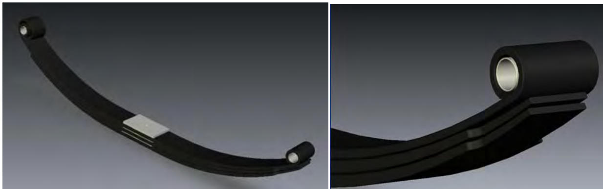
Figure 12. Three-dimensional rendering of the leaf-spring suspension for a Freightliner FLD 120 tractor
