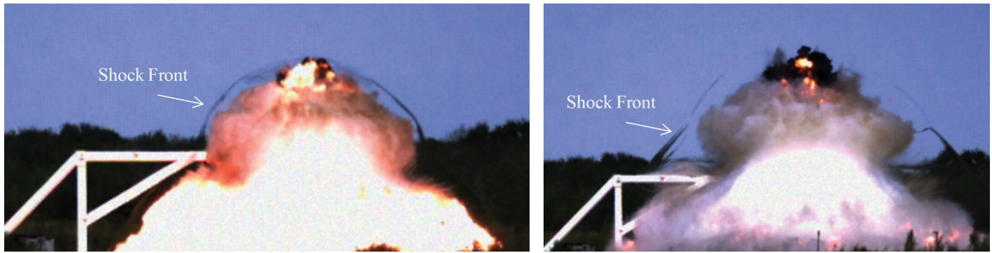
FIGURE 2 Illustration of fireball and shock front from high-explosive detonation.
