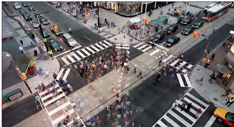
Exhibit 7 – Time lapse of a pedestrian scramble phase over a 24-hour period in Toronto, Canada ( www.spacing.ca ).
