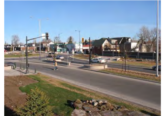
Figure 3. Example of Off-Set or Staggered Crosswalk Condition
