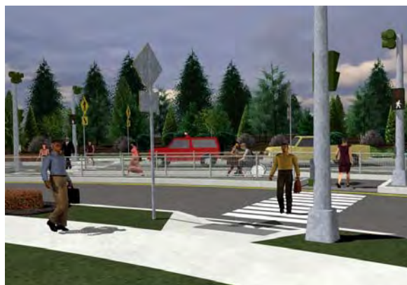
Figure 10. Pedestrian View at Entry Lane of Off-Set Crosswalk Using HAWK Signal and Pedestrian WALK/DON'T WALK Signals
