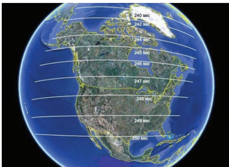
FIGURE 2-7 Thrust cutoff time contours for a notional two-stage liquid ICBM with a maximum nonrotating Earth range of 13,300 km that is launched from central Iran.
