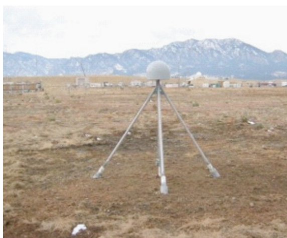
FIGURE 3 GPS Antenna at Marshall, CO PBO site used for soil moisture and snow experiments. Source: Larson et al., 2008a. Courtesy UNAVCO.
