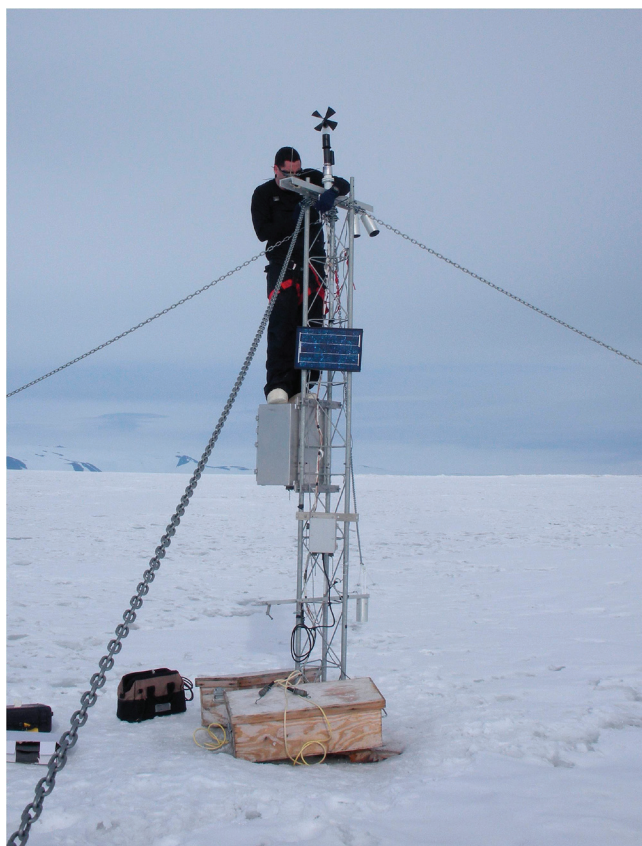
FIGURE 4.11 John Cassano working on an automatic weather station. AWS networks in place during IPY helped fill gaps in surface weather observations. SOURCE: John Cassano, University of Colorado Boulder.
