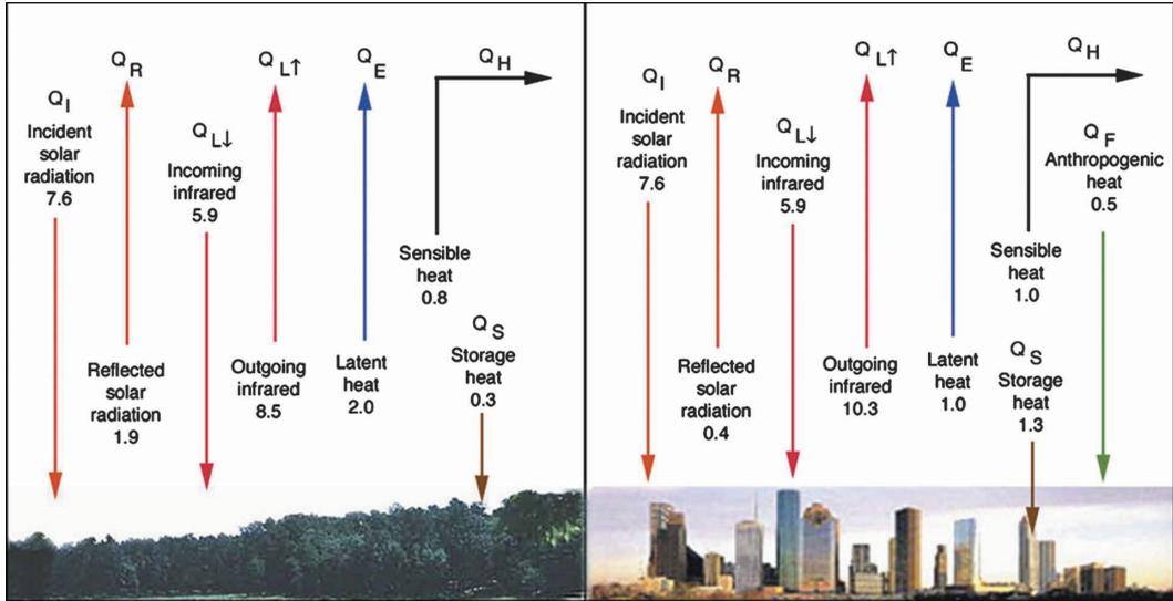
**FIGURE 3.4** A qualitative description of typical rural and urban surface energy balance processes. The values are in units of  $\text{kW h m}^{-2} \text{ day}^{-1}$ . Figure courtesy of R. Sass, Rice University. SOURCE: Shepherd, 2005. © Earth Interactions. Reprinted with permission.
