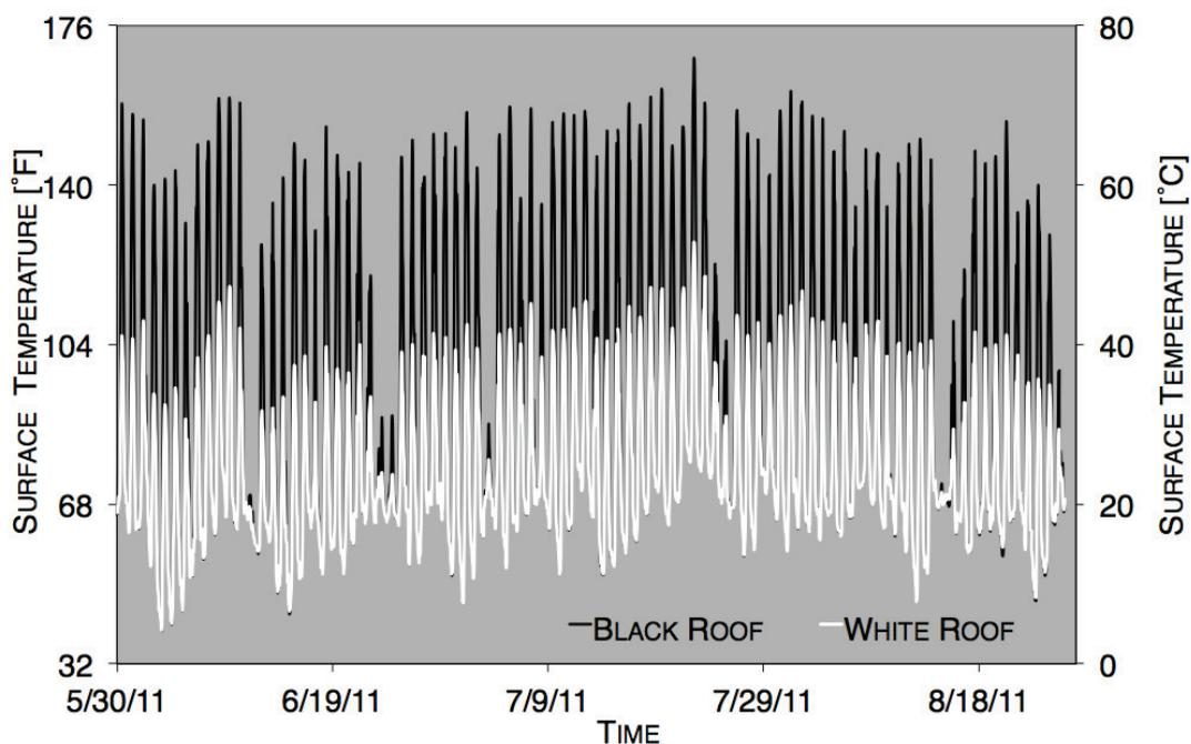
**FIGURE 2.4** The pilot white roof heat island mitigation program in New York City. Results of white vs. black roof surface temperatures. While both colors of roof fluctuate with day and nighttime temperatures, the white roofs stay consistently cooler during the daytime. ([www.nyc.gov/coolroofs](http://www.nyc.gov/coolroofs)) SOURCE: Gaffin et al., 2012.
