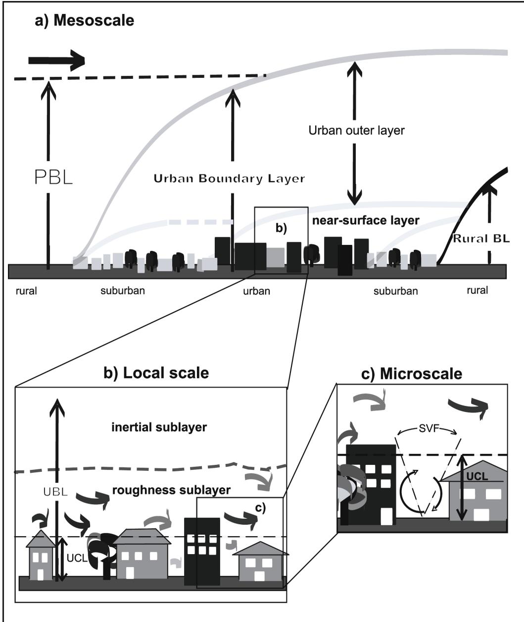
**FIGURE 3.5** Sketch of the urban boundary layer structure indicating the various (sub)layers and their names. SVF in box c) stands for sky view factor. SOURCE: Rotach et al., 2005, modified after Oke, 1987. ©Springer-Verlag Wien. Reprinted with permission.
