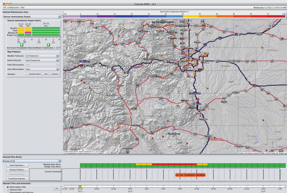
Maintenance and Decision Support System (MDSS) interface—developed from the start with end user input—provides precision forecasts and treatment suggestions to assist managers in making informed decisions on how to best utilize resources. SOURCE: Sheldon Drobot, NCAR.
