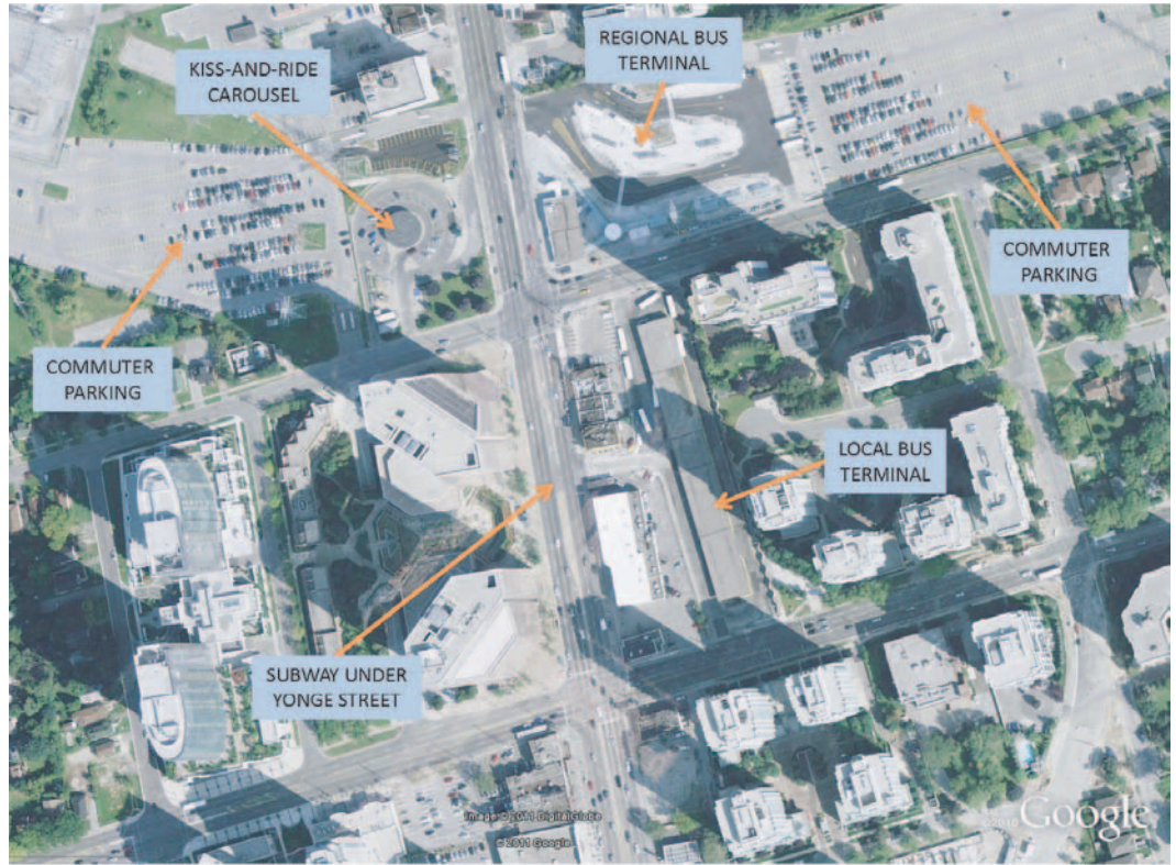
Exhibit 10-15. Park-and-ride lot separated from bus loading and transit platform access (Willowdale, Ontario).
