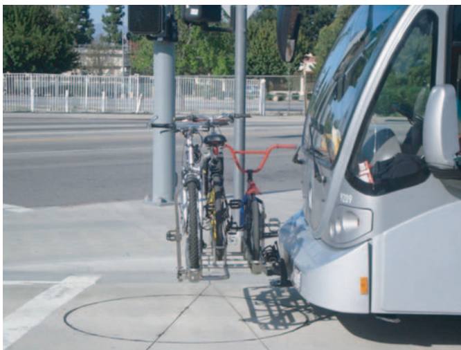
Exhibit 8-6. Exterior bicycle rack on BRT vehicle (Los Angeles).
