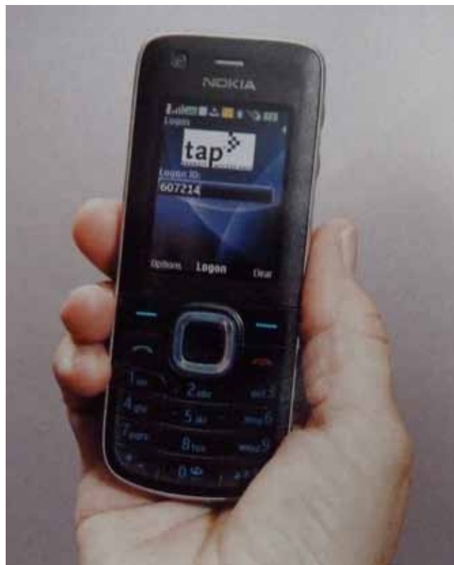
FIGURE 21 Handheld verification device used by LA Metro sheriff's deputy assistants for fare inspection of TAP cards.
