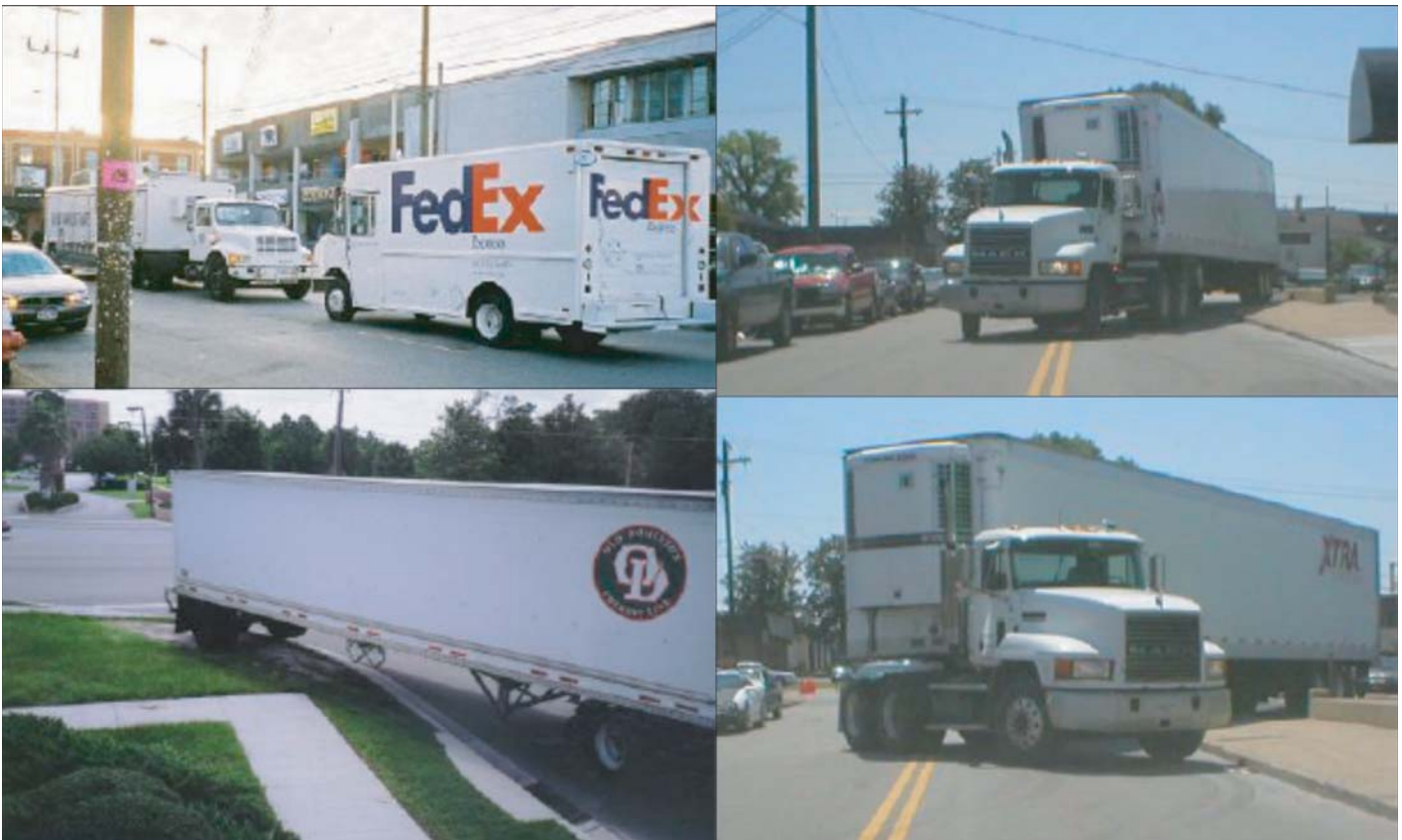
Exhibit 5-4. Urban infrastructure design: inadequate curbside parking and inadequate turning radii at intersections.
