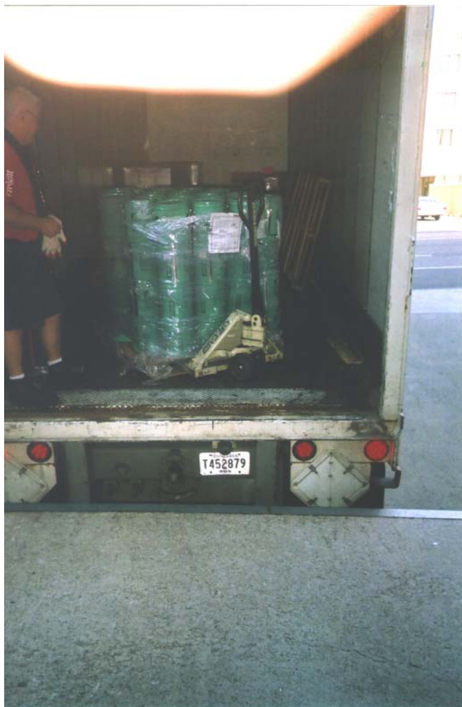
Exhibit 5-3. Docking space with height mismatch (note position of dock against mud flaps).
