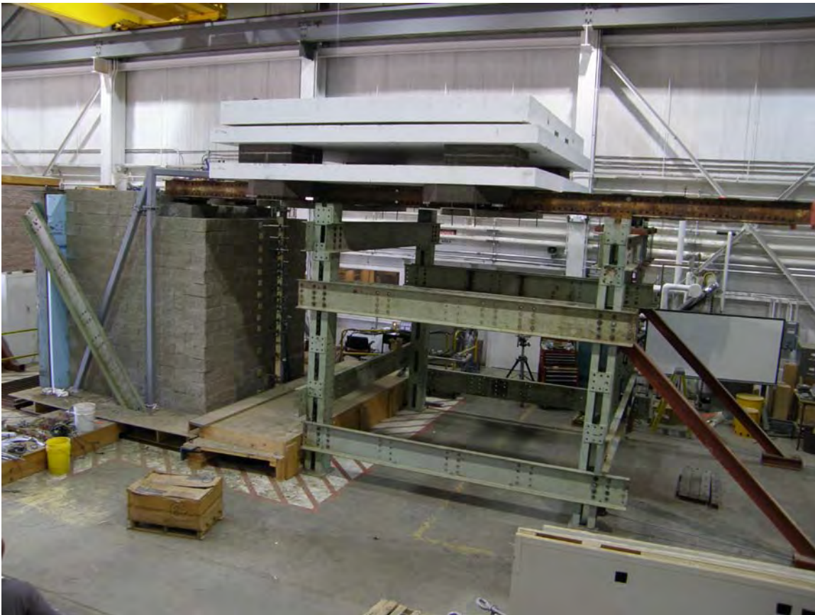
Figure 5.3: Completed Bridge Abutment Model
