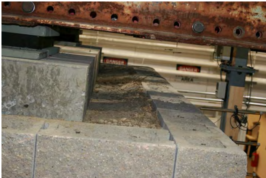
Figure 6.4: Photograph of Sill Movement (Front) after 0.15 g Test at 1.5 Hz
