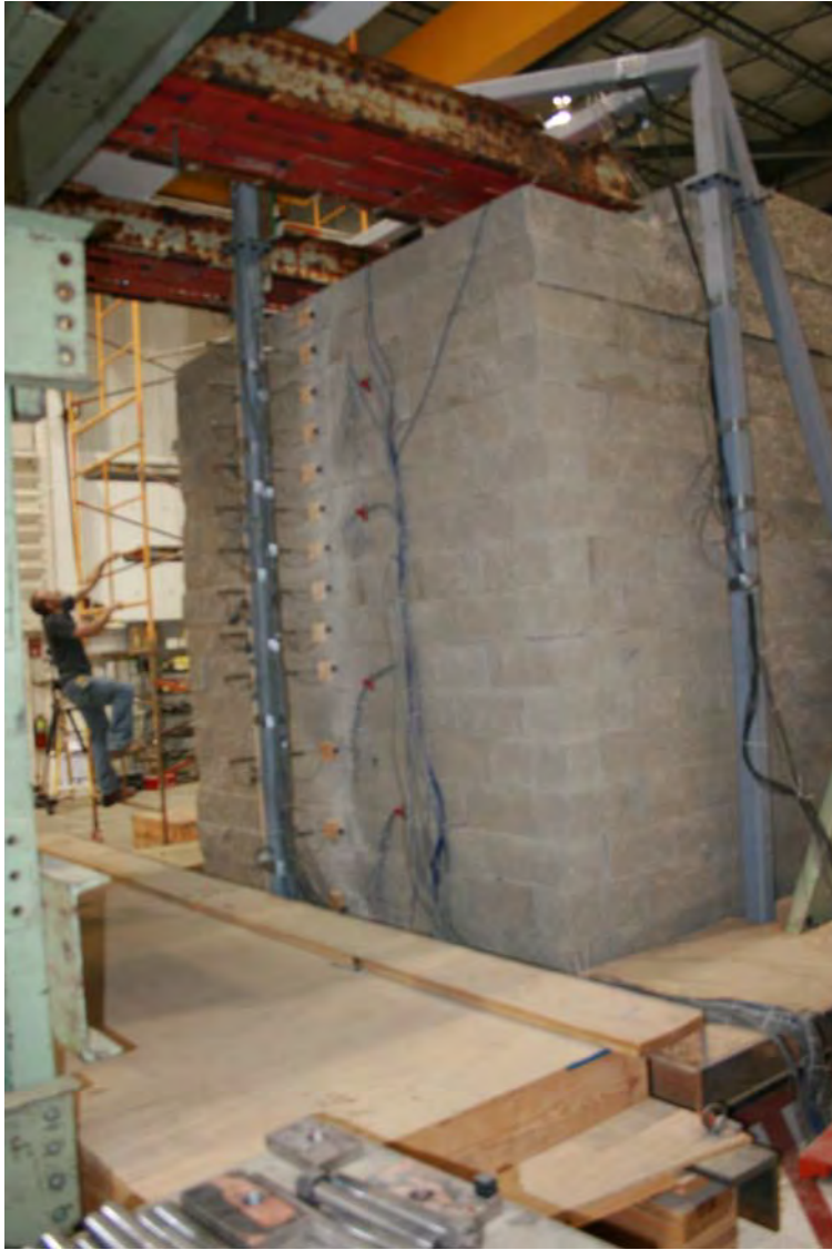
Figure 6.2: Photograph of GRS Abutment after 0.15 g Test at 1.5 Hz
