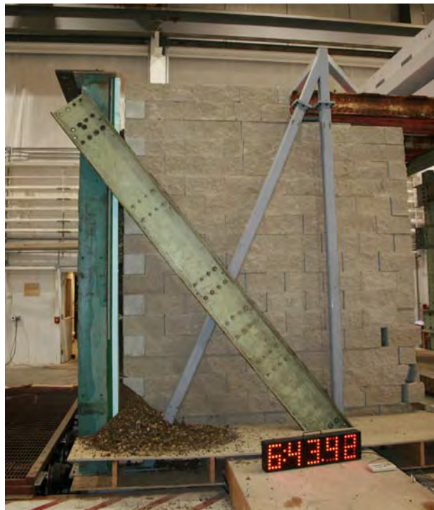
Figure 6.9: Photograph of Abutment Separation from Backwall (Side View) after 1.0 g Test at 3 Hz
