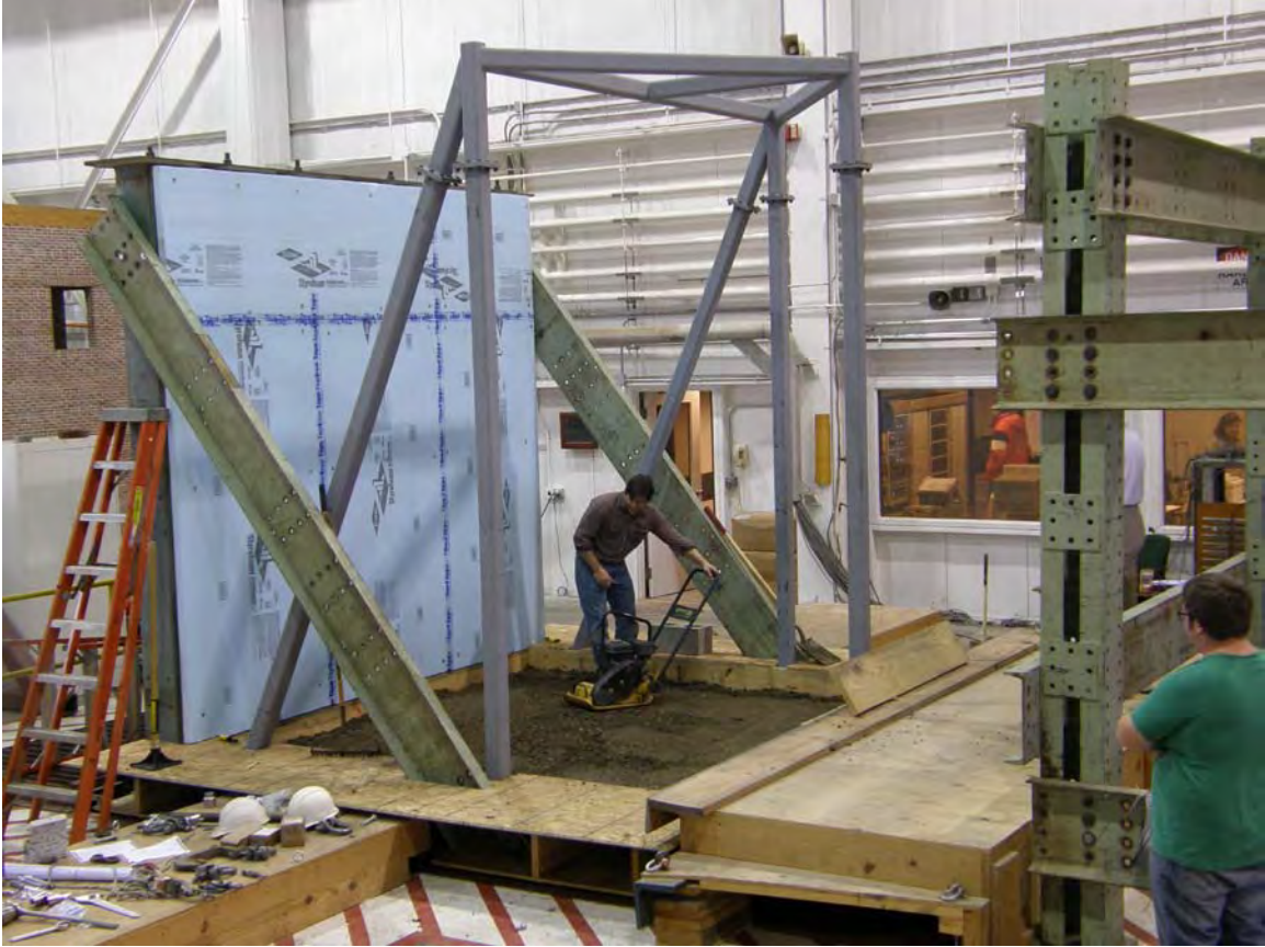
Figure 5.4: Placement and Compaction of the First 10 cm Layer of Soil
