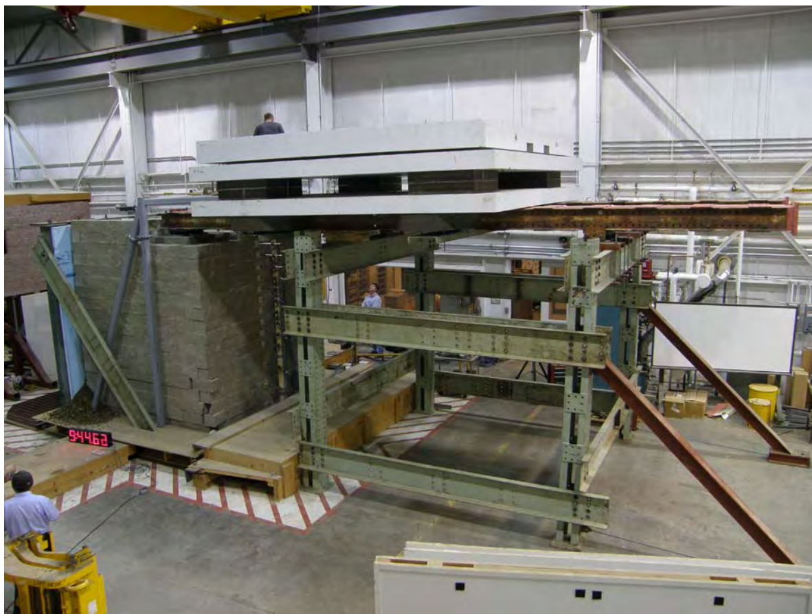
Figure 6.7: Photograph of GRS Abutment and Bridge after 1.0 g Test at 3 Hz
