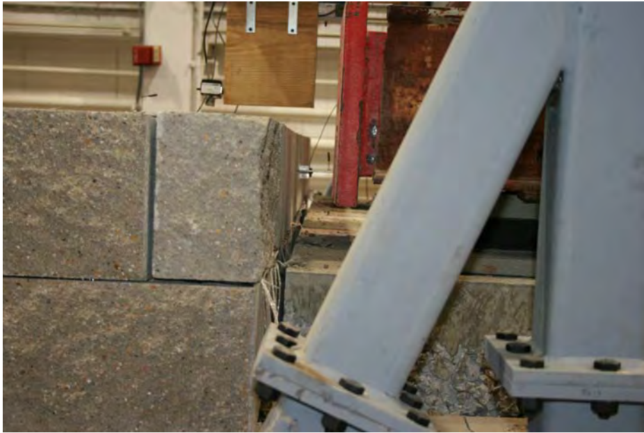
Figure 6.3: Photograph of Sill Movement (Back) after 0.15 g Test at 1.5 Hz
