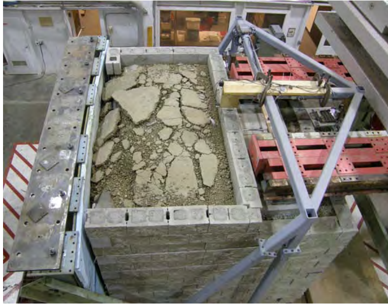
Figure 6.10: Photograph of Abutment Separation from Backwall (Top View) after 1.0 g Test at 3 Hz
