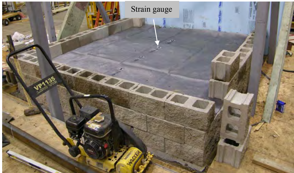
Figure 5.13: Strain-Gauge Instrumented Geosynthetic Layer Placed Above 2 nd CMU Course
