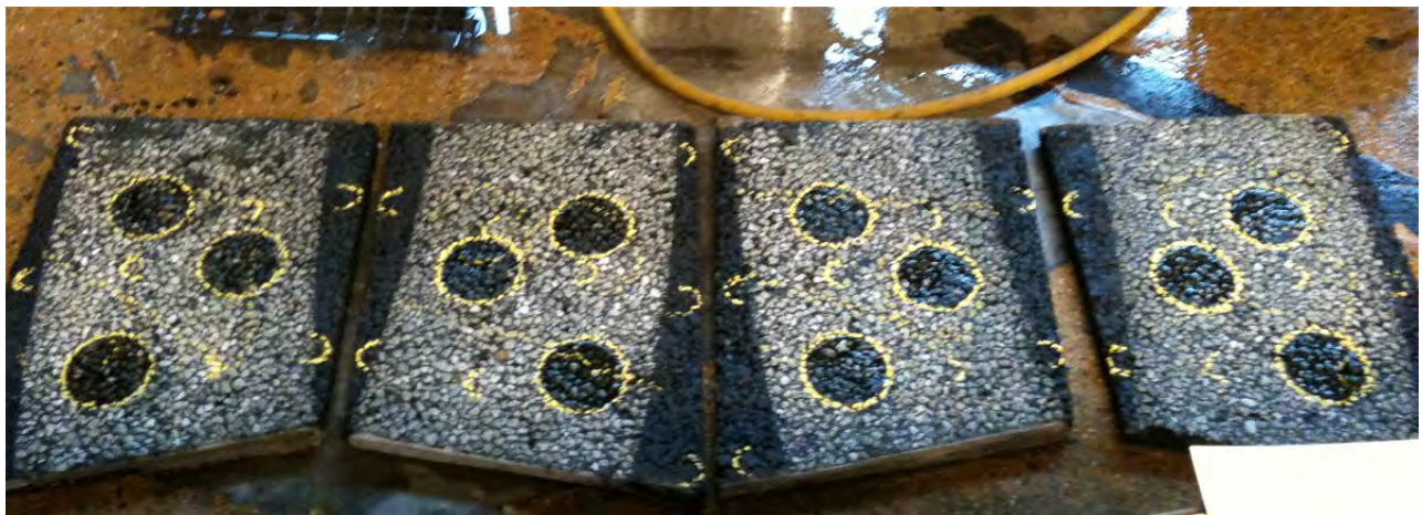
FIGURE 1 Asphalt slabs used for comparison of salt measuring field techniques.
