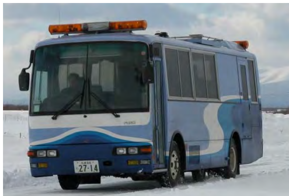
FIGURE 2 Bus-type locked-wheel friction tester.
