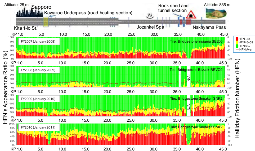
FIGURE 7 Appearance ratios of road surface conditions (friction) on National Route 230 during January of 2008, 2009, 2010, and 2011.
