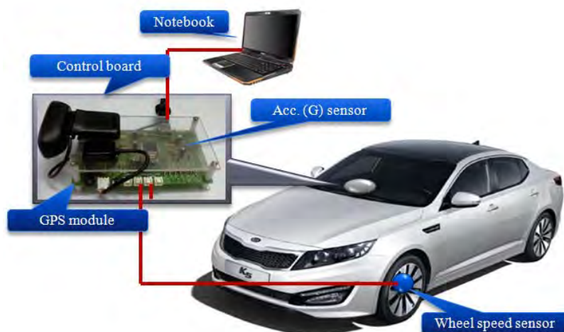
FIGURE 1 Data collection devices applied to a probe car.
