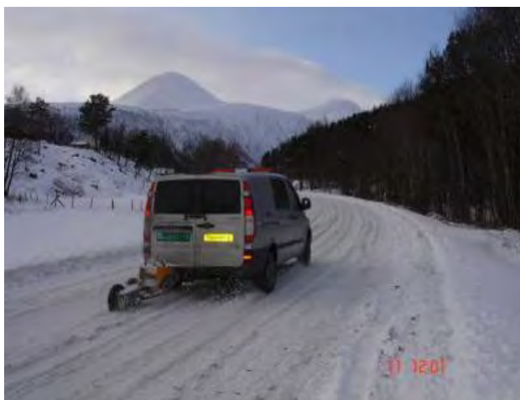
FIGURE 10 Friction measurement with a TWO-type friction trailer.
