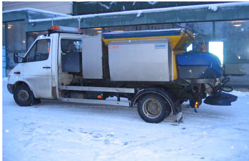
FIGURE 1 The equipment used for spreading warm wetted sand on walkways and bike paths in Umeå municipality, in Sweden.
