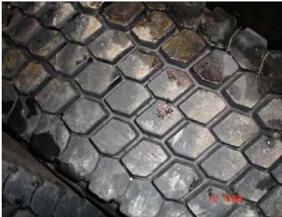
FIGURE 8 "Foreign" block pattern tire. Shore value: 72.
