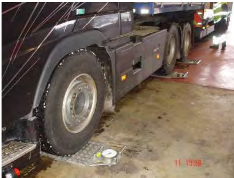
FIGURE 9 Setup for weighing with mobile scales.
